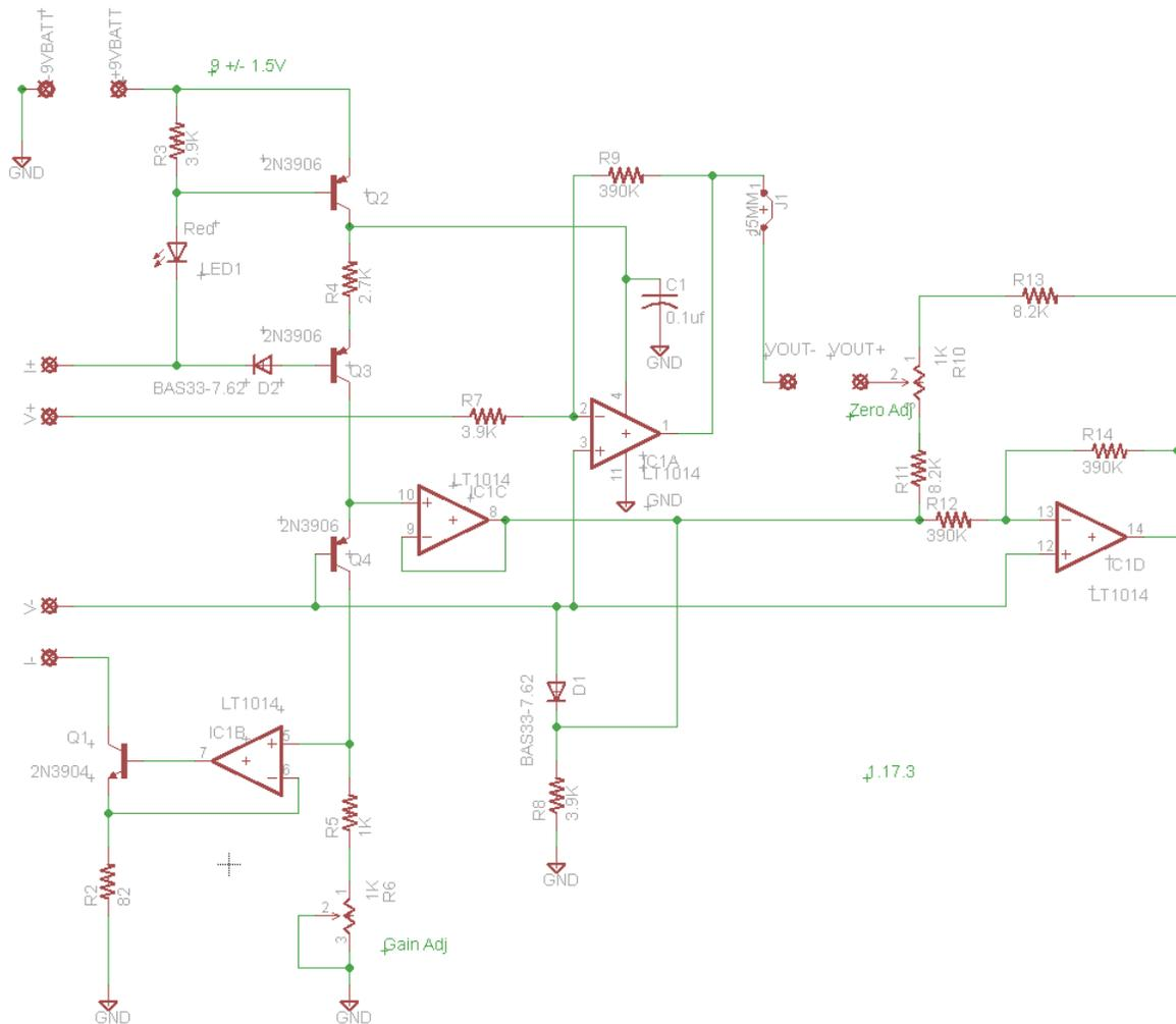
When Q2 is saturated and the LED is on, a voltage is developed across R4. This causes a current to flow into the emitter of Q3 and about 98% of it flows out of its collector. This collector current then flows into the emitter of Q4 and about 98% flows out the collector. The Q4 collector current flows through R5 and trim pot R6 to define the voltage at pin 5 of op amp B. This voltage is then applied across R2.
