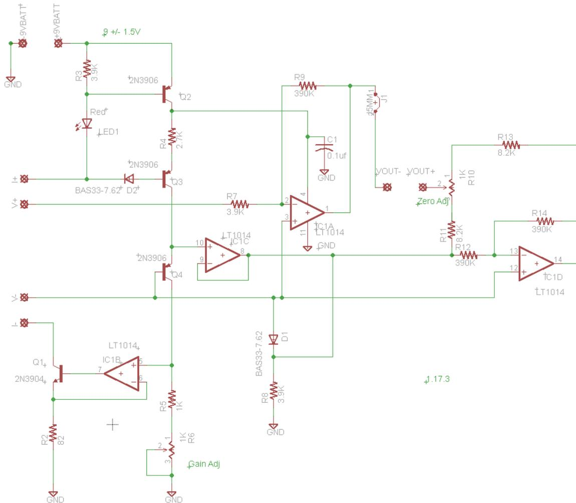
Power is controlled by Q2 which senses when the test current is flowing out of the I+ lead. When this current is present, Q2 saturates and LED1 lights. It then applies power to the quad op-amp IC.
