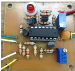
The circuit must first have the two black clips (I- and V-) connect to the unknown resistance and then the two red clips (I+ and V+) connected. Connecting in the wrong order causes the LED to be dim and the voltmeter to read negative.
