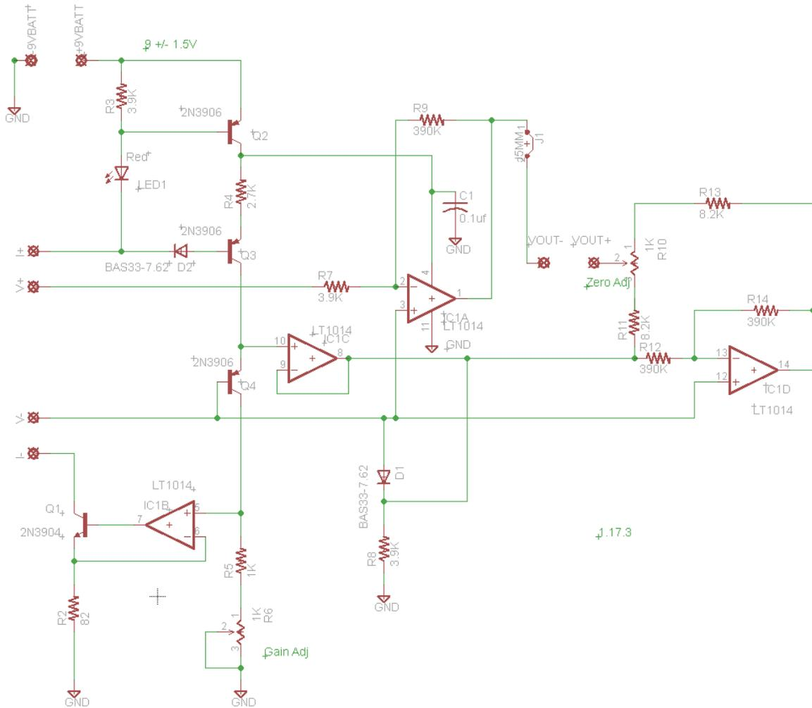
I used a 22 turn trim pot which means one full turn causes a change of about 3 mV. It is therefore rather easy to adjust it to within 1 mV of the desired value.
