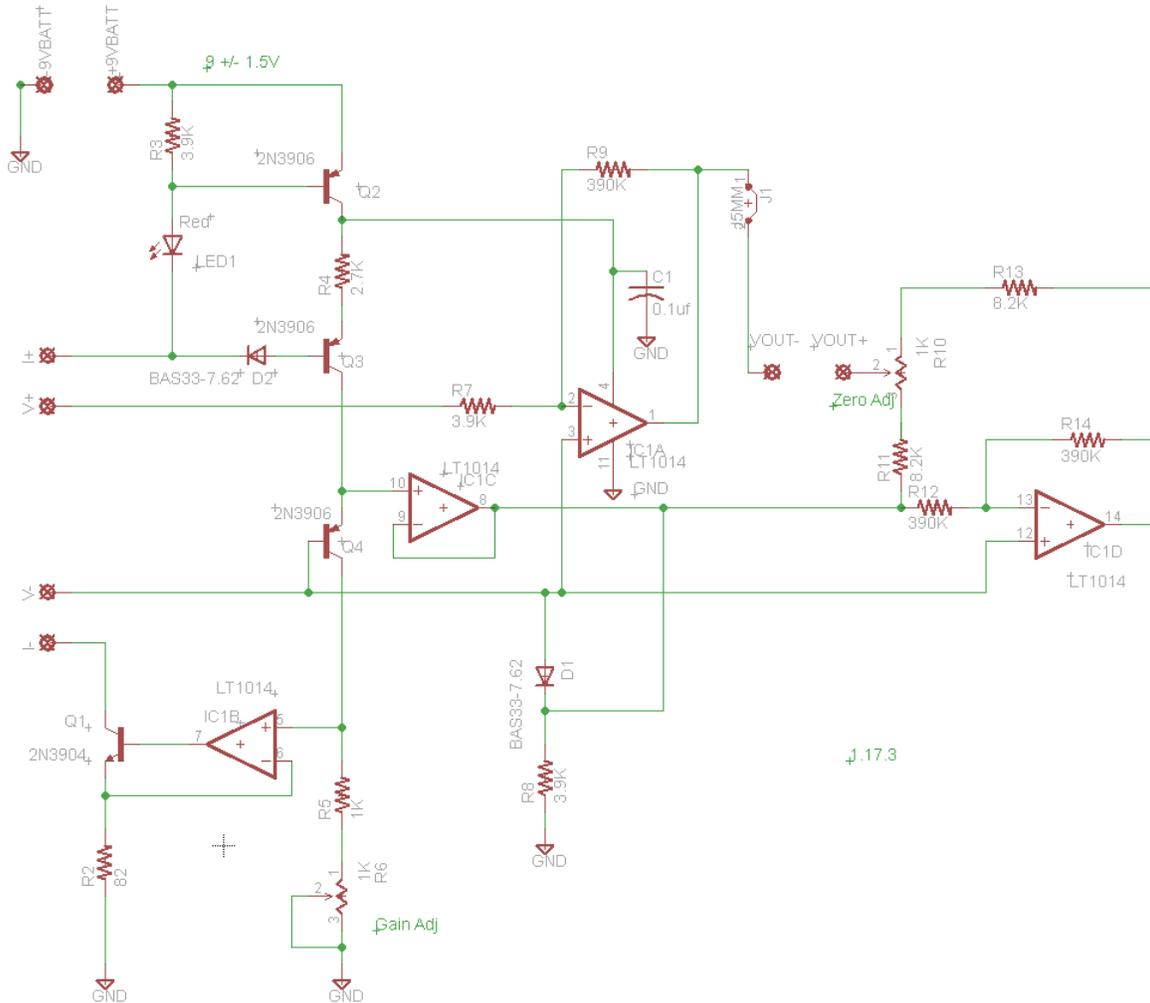
The worst case variation in gain is - 90 to -110 or  $\pm 10\%$  because I am using 5% resistors.
