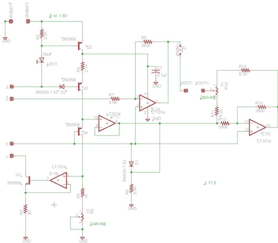
Going back to the power and current source circuit, you can now see that Q4 passes the current coming from Q3 which is set mostly by the voltage across the LED and D2. Since the current through Q4 is stable, its voltage will only be a function of temperature. Variations in battery voltage have a minimal effect.
