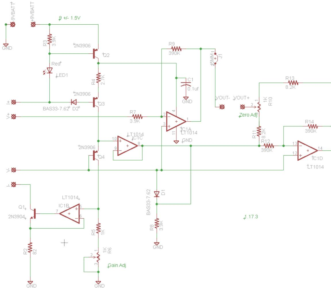
You will see in the next section that  $V_{out+}$  is just a DC voltage that cancels the offset present in  $V_{out-}$ . Therefore, I can assume this adjustment has been made and say
