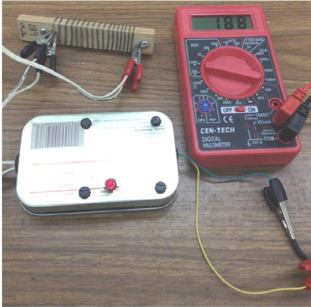
Most Digital Volt-ohms-Meters (DVMs) can measure down to 1 ohm. But what if you want to measure smaller resistances, say 0.001 ohms? This can be useful if trying to find a short on a circuit board or for measuring the electrical resistance of bearings in order to select the proper Lathe Electronic Edge Finder model. This article details a low cost device that amplifies the unknown resistance so a common DVM can measure it. Call it a Resistance Amplifier.
