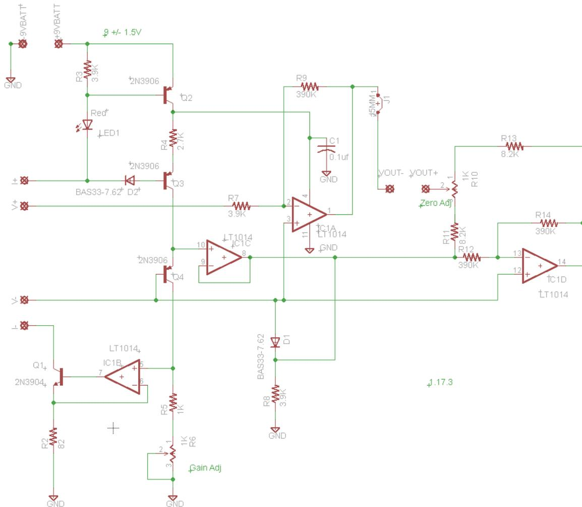
This test current passes through the unknown resistance to generate  $V_x$  which feeds the voltage amplifier
