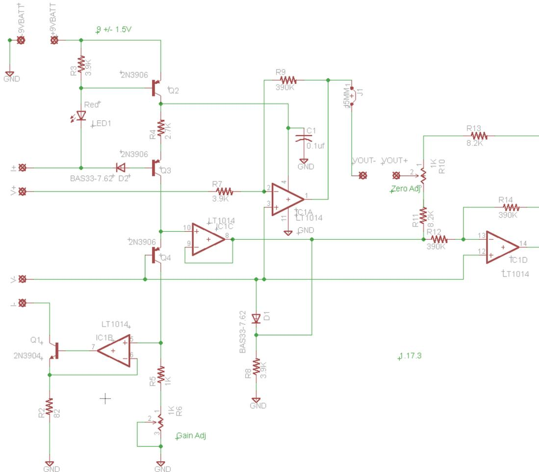
When the circuit is first starting up, the current out of the I+ node is less than the full amount. This current is
