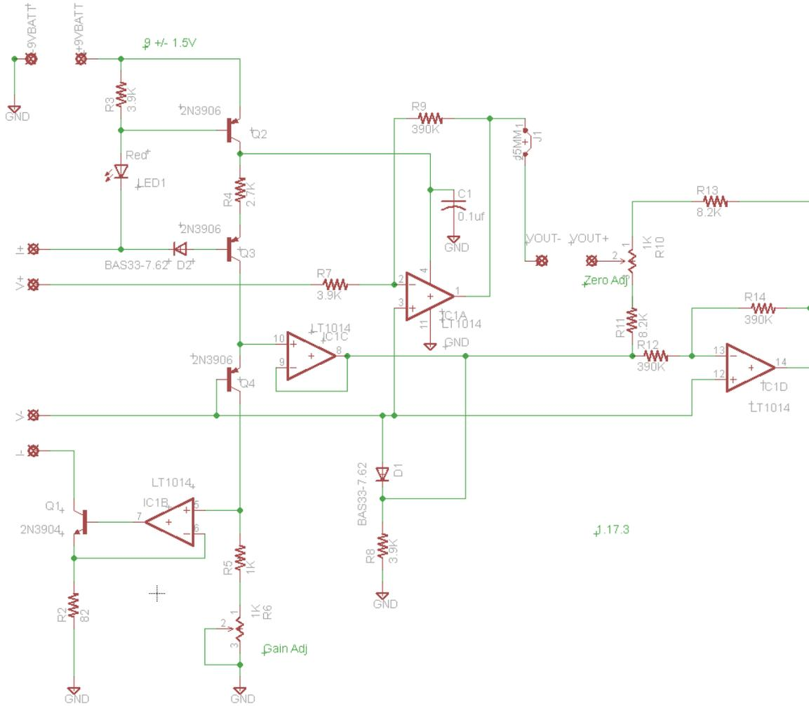
The worst case offset voltage at  $V_{out-}$  is canceled by the voltage at  $V_{out+}$ . The voltage divider string formed by R10, R11, and R13 is fed by  $V_8$  and  $V_{14}$  which are outputs of op amp C and D respectively.
