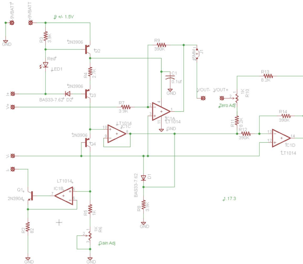
Although the quad op amp LT1014 is very good, there is still up to  $\pm 0.3$  mV of input offset voltage present. With the amplifier set for a gain of  $-\frac{R_{11}}{R_{10}} = -100$ , this means that the output can be  $\pm 30$  mV due to input offset. If ignored, this would contribute an uncertainty in the output equal to the equivalent of  $\pm 30$  m $\Omega$ .
