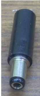
Note that I did not use the black shell that came with the male connector. I wanted to have this connector body stick out of the laptop as little as possible.
