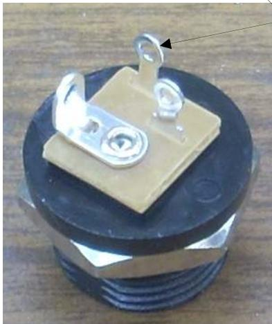
There is a third tab that connects to the outside contact only when the jack does not hold a male connector. I just cut that tab off.
