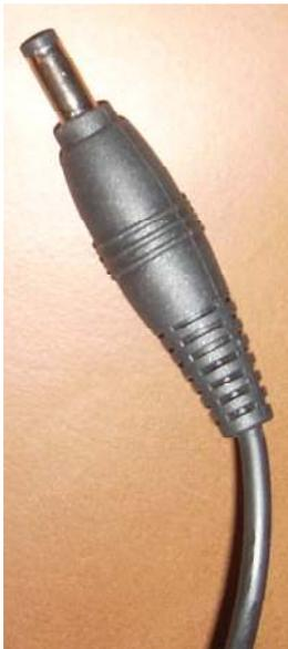
The power plug has a massive strain relief on it. This strain relief protects the low cost power cable from pulling out of the low cost plug.
