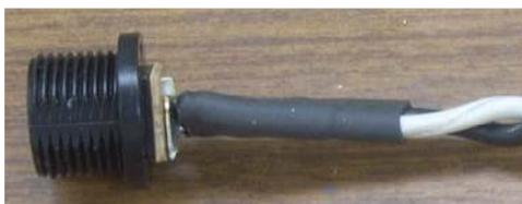
As a final step, I slid a piece of black heat shrink tubing over the wires. I don't mind these wires breaking. I just don't want them shorting out.
