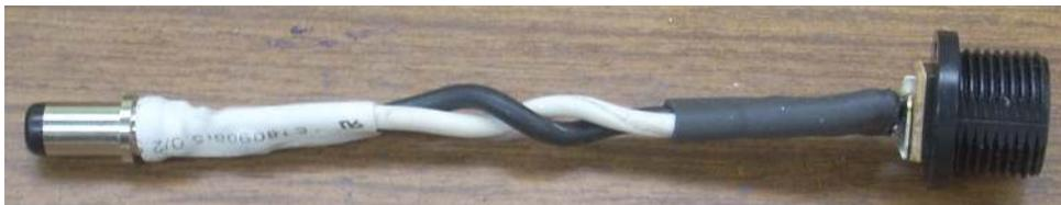
After both wires were soldered to the male connector, I slid down the
