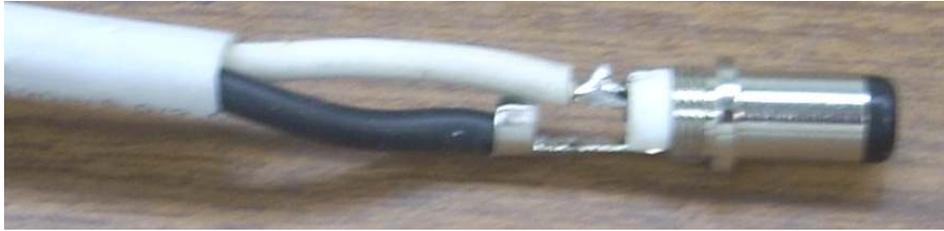
I slid on a piece of white heat shrink tubing before attaching the wires to the male connector.
