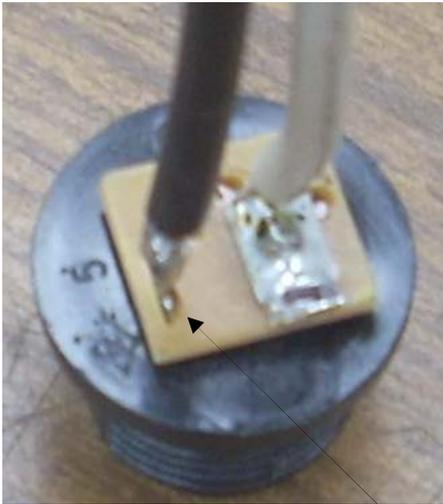
Here you see the white wire soldered to the central pin of the female connector. The black wire connects to the outside contact. I trimmed off the excess tab on the central pin connection.
