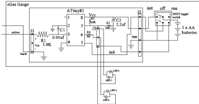
I now have independent control of LED1 and 2 at all times. When not in Initialization, I have independent control of all four LEDs.
