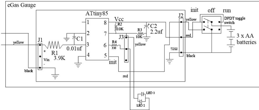
I connected LED1 and LED2 back-to-back. One end connected to pin 6 by way of R4. The other end is connected to pin 7.
