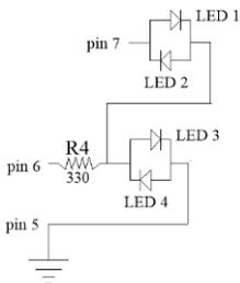
When pin 6 is high, I can turn on LED3 if pin 7 is an input. If pin 7 is low, LED2 and LED 4 would be in parallel. There would be no way to control how the current flowing in R4 would split between them. If pin 7 was high, LED1 would be in series with LED3. This would likely put pin 7 in overload. Not good.
