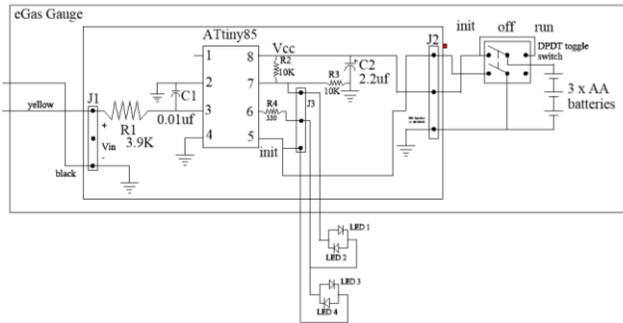
As wired, pin 5 is grounded during Initialization and left open the rest of the time.
