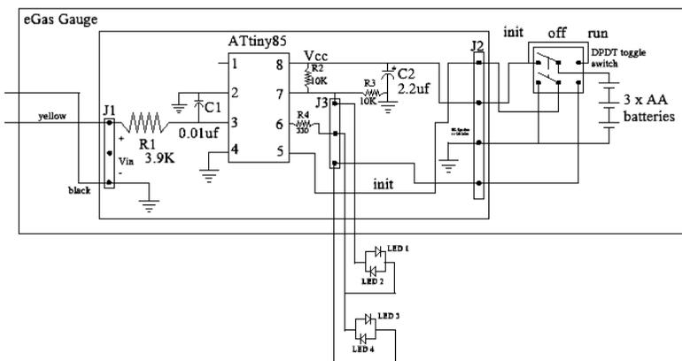
All is not lost. I can rewire the switch. When in Initialization, pin 5 still sees ground, but now LEDs 3 and 4 are not connected. This lets me control LED1 and LED2, which does meet my needs.
