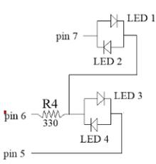
I could turn LED1 on by setting pin 7 high, pin 6 low, and pin 5 as an input.
