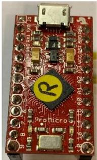
Don't get me wrong, Sparkfun's 5 volt, 16 MHz Pro Micro<sup>2</sup> is a terrific product. I use them in almost every one of my Arduino compatible applications. Most of the time, I have a simple system with just one Pro Micro and a few external parts. But once in a while it can get a bit more complicated. This is where I often run into the Pro Micro's design defect.
