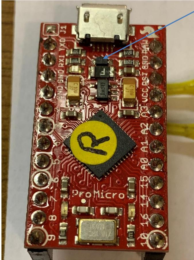
First, let's look at the culprit. As with most surface mount components, it is crazy small. Given a steady enough hand and a fine enough point on my soldering iron, I might be able to desolder it.
