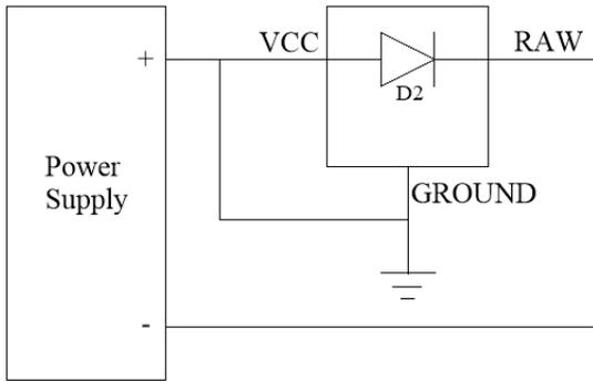
If you are using a power supply that will limit the current to under 2 amps, connect the positive lead to the Vcc pin on the Pro Micro. Also connect a ground pin on the Pro Micro to Vcc<sup>7</sup>. The negative lead connects to the pin marked RAW.
