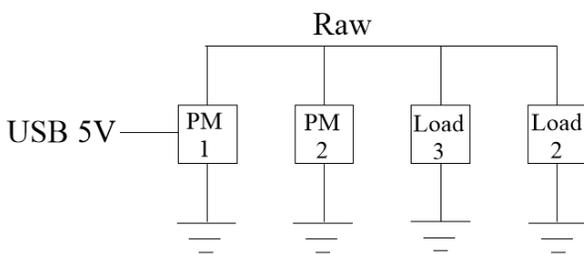
I plug a USB cable into the first Pro Micro. Funny things start to happen with the second Pro Micro and the two loads. They sort of turn on but not fully. I might even find that the first Pro Micro is not acting correctly. It may not be getting a supply voltage above the minimum limit. What is going on?
