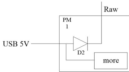
Look inside a 5V/16 MHz Pro Micro and you will find this diode, D2. When you plug in a USB cable, 5 volts from the cable is applied to the anode of this diode. The cathode connects to the Raw input but now Raw is an output.
