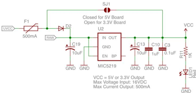
UVCC is the voltage from the USB. Since this is a 5V board, jumper SJ1 is closed. This lets us power the board directly from the USB<sup>3</sup>.
