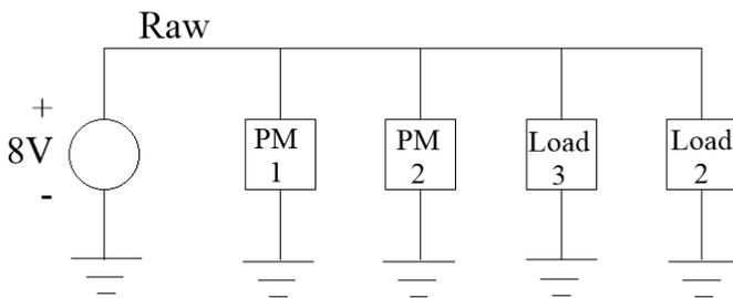
Consider this system. I have an 8V power source that feeds two Pro Micros plus two other loads. Works fine. Well, until I want to program one of the Pro Micros.
