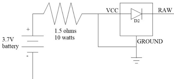
If you are using a 3.7V battery and a 1.5 ohm resistor, connect the positive lead of the battery to one end of the resistor. Connect the other end of the resistor to both Vcc and ground pins. Connect the negative lead of the battery to RAW.
