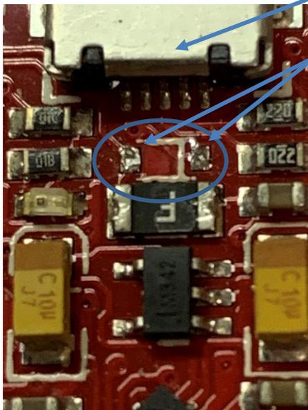
the USB connector with the toothpick. The instant you push either end of the diode off of its contacts, current will stop flowing and the solder will start to cool. It is likely that one end of the diode will remain soldered while the other end is free. You can leave it this way or pry it up with the toothpick to remove it.
