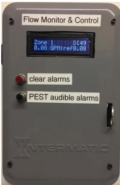
This package of hardware and software is able to stop water wasted due to irrigation leaks. Within one minute, it will detect and shut down any zone with a flow rate greater than 30% above normal. Besides sounding an audible alarm, it sends an email to the user<sup>2</sup>.
