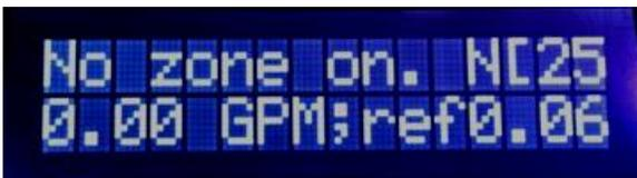
When no zones are on, the flow is compared to a limit<sup>4</sup> of 0.06 GPM. Flow less than 0.06 GPM is considered acceptable.
