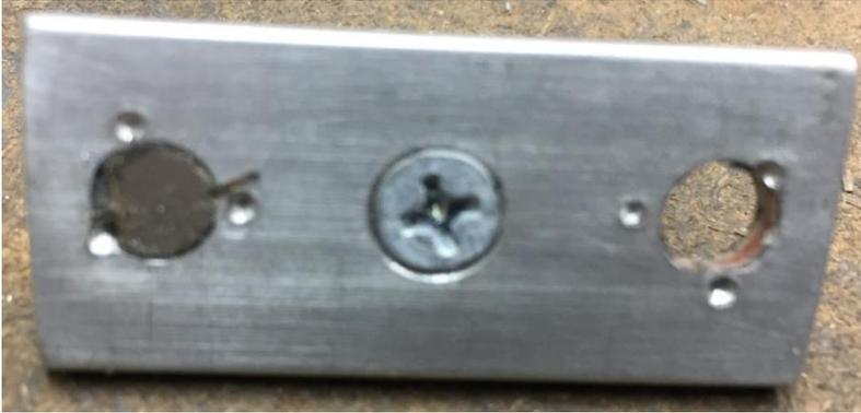
I locked it in place with 3 punch marks. At first I had two magnets but found that this prevented movement.
