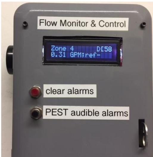
When either of the pushbuttons is depressed, a contact closes and the port expander sees a logic 0. When released, the internal pull up resistor generates a logic 1.
