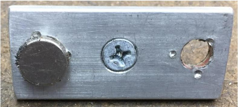
I later found that I needed to move the bar closer to the top of the meter in order to insure reliable coupling. Placing a 3/8 inch diameter by 1/8 inch thick magnet on top did the trick.
