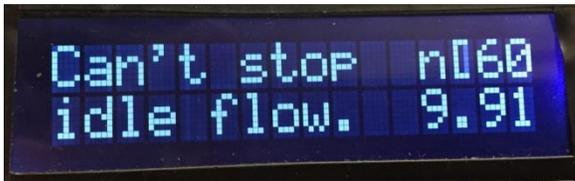
When no zones are on and the flow exceeds the limit of 0.06 GPM, we get an Overflow condition and a Major Alarm is sounded both day and night. It will sound for 0.1 seconds and be quiet for 0.1 seconds. The number in the lower right hand corner is the current flow. It is possible to see "Can't stop idle flow." with a current flow of 0. This means it *was* greater than 0.06 GPM but is *now* zero.
