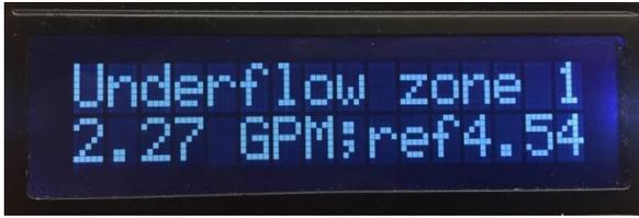
If the flow is more than 30% lower than the threshold, we get an Underflow condition. The second line shows the current flow and normal flow (ref). If during the day, a Minor Alarm is sounded.
