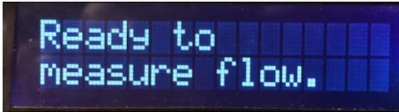
The FMC can be turned into a flow meter by holding down the PEST button when power is off, turning on power, and then releasing the button. Power cycle the FMC when done measuring flow.
