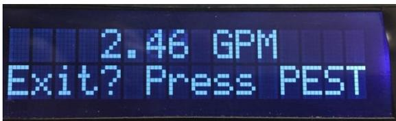
Once a non-zero flow rate is measured, the display will update every second. If the flow returns to 0, the last non-zero flow rate will remain on the screen. Press the PEST button to return to normal flow monitoring behavior.
