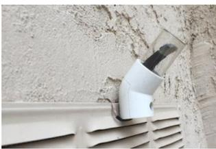
My light sensor is mounted inside a glass bottle that is a tight fit into a PVC 45° coupler. I happen to have two wire speaker cable. Since the ALS-PT19 has three terminals, I would need to run two of these speaker cables and have half of one cable unused.
