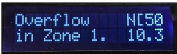
If the flow is stopped, the screen indicates the problem. If it is daytime, the Flow Monitor and Control sounds a Minor Alarm which is 0.3 seconds on and 2 seconds off. The flow that triggered the alarm is in the lower right corner.
