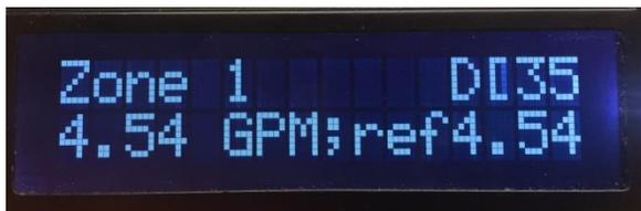
It is also common to see the flow rate on the second line. Here you have 4.54 GPM. It is being compared to the reference which is also 4.54. If there was no reference yet, you would have seen "ref-". After the zone has
