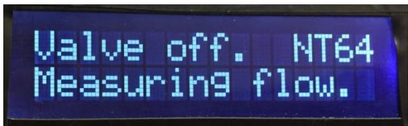
If the new flow is more than 30% higher than the reference, we get an Overflow condition. The system responds by turning off the valve and taking another flow measurement.
