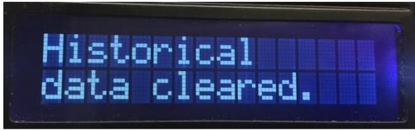
If the clear alarms button is held down before power up<sup>6</sup> and released after power up, all historical data will be erased. The system will then collect new data as the zones turn on and off.
