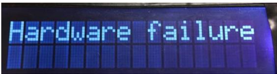
There is an electromechanical relay inside the Flow Monitor And Control that can fail. As long as it is stuck in the open position, this message will display and a Minor alarm will sound. However, if the problem goes away, we will return to normal operation.
