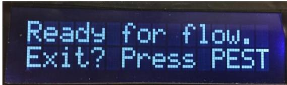
If the PEST button is held down before power up and released after power up, you will see the current instantaneous<sup>7</sup> flow rate. Before any flow is detected, you get this screen. Press Clear Alarm at any time to return to this screen.
