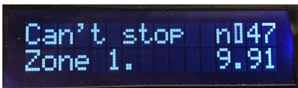
If the Flow Monitor and Control was unable to stop the flow<sup>5</sup>, the screen tells the story and a Major Alarm is sounded. The current flow is in the lower right corner.
