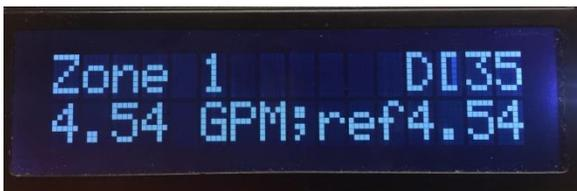
When a give zone is run again, its flow rate is compared to the reference. In this case, the current flow matches the flow the last time this zone ran.
