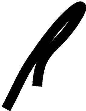
One way to detect leaks in a zone is to block all  $\frac{1}{4}$  inch lines and see how much flow is left. This can be done by bending each  $\frac{1}{4}$  inch line in half and securing it with a piece of wire or bag tie. No water should then come out of the emitter. With all  $\frac{1}{4}$  inch lines blocked, the flow seen by the FMC will be from leaks.
