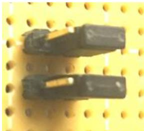
Not shown in the diagram are two jumpers that can simulate Zone 1 and Zone 2 being active. Here you see both jumpers set to normal operation.
