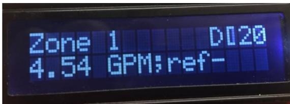
When The Flow Monitor and Control is first powered up, it records the average water use for each zone. Here you see Zone 1 is active and the flow is 4.54 Gallons Per Minute (GPM). These measurements are saved as the first reference
