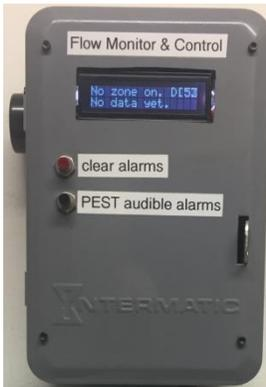
The second piece of the puzzle is the Flow Monitor and Control that will read the flow signal from the water meter plus read and control the signals in the cable. This intelligence will have control of the valves including overriding the Irrigation Controller if a fault occurs in the valves or irrigation zones.
