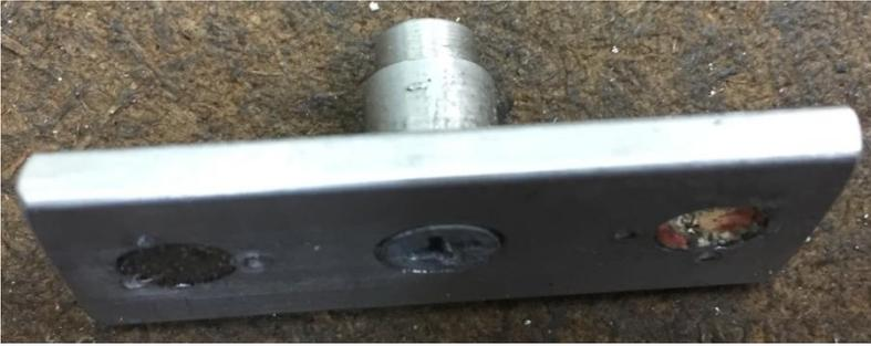
The bar has a spigot on the back that is a close fit to the ID of a ball bearing. The bar has a 1/4 inch diameter hole in it that accepts a neodymium magnet 1/8 inch thick.
