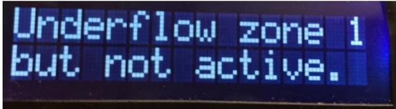
If the underflowed zone is not active, the system will monitor and control the other zones while displaying the error message for the faulted zone.
