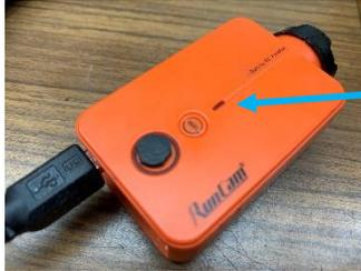
If all goes well, this blue bar will start to flash. If it doesn't, quickly push and release the power-on/shutter button again and then push and release the Wi-Fi button. Hopefully, it will now be flashing. I often ran into this annoying intermittent behavior with the camera and app but, once configured, all was solid.
