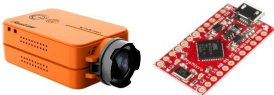
The challenge was to have a RunCam2 camera<sup>2</sup> fully controlled by an Arduino based Pro Micro<sup>3</sup>. I also needed to have the camera power up when the Arduino received power.
