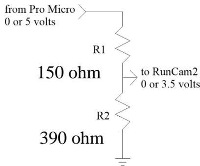
The solution involved configuring two resistors as a voltage divider. A Pro Micro digital output connects to the top of R1 and the RunCam2’s green control line connects at the junction of R1 and R2. Both resistors are +/- 5% and have a power rating of 0.1 watts.
