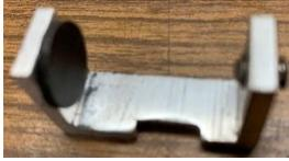
The clamp was made from a piece of aluminum extruded channel. The lower clamp face was lined with a disk of stick on rubber. The upper clamp face was drilled and tapped for a 10-24 set screw. That notch was needed to clear the USB connector.
