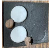
The disk on the button's face was cut using a 1/4 inch diameter paper punch. The lower clamp face's 1/2 inch diameter disk was precut on the sheet.
