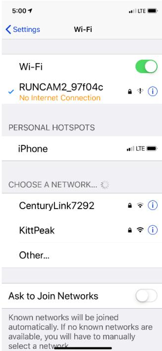
With the blue bar flashing, go to iPhone's Settings and select Wi-Fi. The RunCam2 will be broadcasting a host signal just like your router. Select RunCam2 and wait for the password prompt. The default password is 1234567890. Hopefully, that works for you.
