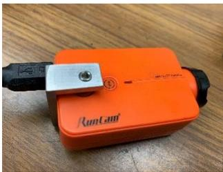
The clamp is placed around the camera and the set screw turned until you can hear the button click. Overtightening this screw can damage the camera.
