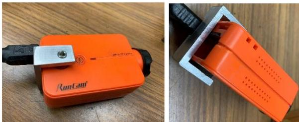
Instead of an electromechanical device to push and release the button, I just needed a simple clamp to hold the button down.
