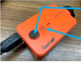
The first step was to power up the RunCam2 by pushing the power-on/shutter button for about 3 seconds. Then I released the button.
