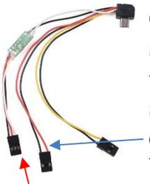
One piece of the puzzle was a RunCam2 Remote cable<sup>4</sup> which takes the slow toggling of a digital line (red arrow) and somehow gets the RunCam2 to switch between video and still. It also will start and stop video or take a single still picture. External power is supplied to the RunCam2 by the connector with the red and black wires. RF output<sup>5</sup> is on the yellow and black wires.
