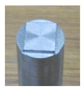
But then I realized that I could directly measure the width of the slot on the lower guide which would give me a more accurate value. It turned out to be 0.606" so I change my cutter to 0.303" and took the cut. Rotating 180°, I took my last cut.
