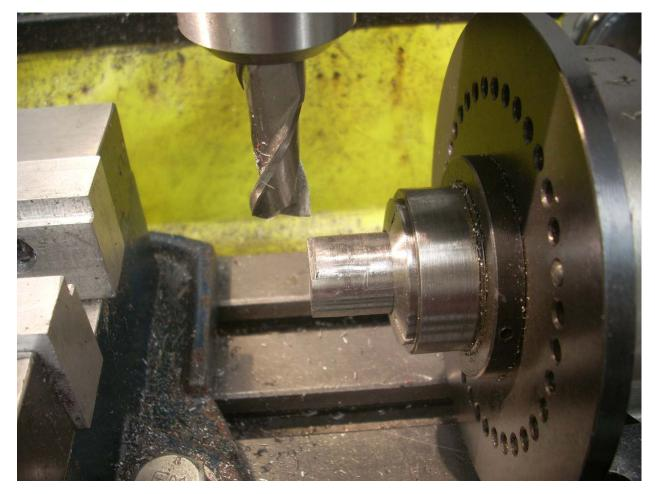
The  $\frac{3}{4}$ " bar is clamped in position and the indexer locked at 0°. I then touched the cutter down on the top surface of the work piece, zeroed it, moved it away from the bar, then lowered the cutter down 0.375". I then zeroed the Z axis again. My zero point is now at the center of rotation of the rod. I then raised it up 0.250" and fed in 0.055" to set the width of the cut.
