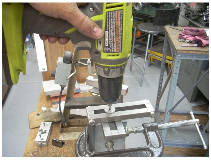
I used my hand held electric drill with an 1/8" drill. The guide was solidly in place.
