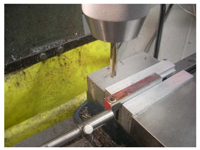
After using my spotting drill, I ran my #7 drill in preparation for tapping. I then chucked up a spiral point <sup>1</sup>/<sub>4</sub>-20 tap. Then I squirted in some cutting oil.
