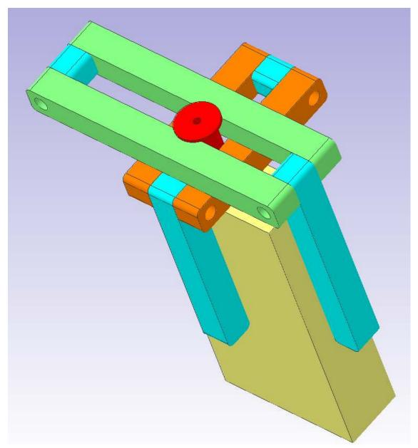
This rendering lets me explain the operation of the guide plus how to best make it. The guide requires that the end of the work piece be perpendicular to its major axis. Those two orange bars contact this reference surface plus permit the bushing to slide between them. Similarly, the two green bars contact the tops of the orange bars plus permit the bushing to slide between them.
