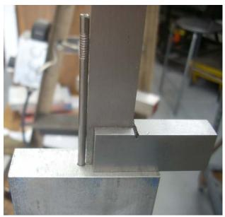
I could not find a close fitting rod to test the alignment of the hole. Here I used a nail but it turned out to be slightly bent. So all I can say is that the hole looks fairly straight...
