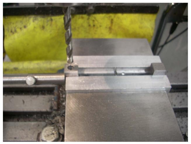
Drilling the spacer blocks required some packing material on the right end of the vise jaws to insure that the movable jaw made square contact with the block being drilled. After finishing the block on the left, I swapped the two blocks and processed the second spacer block.
