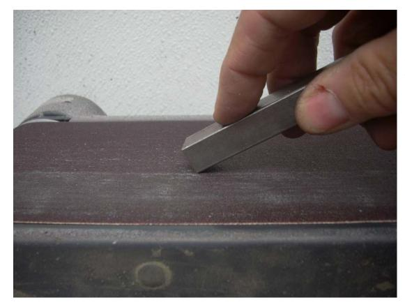
Each piece is carefully deburred and then cleaned with alcohol.
