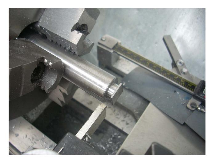
I used my 3/16" wide parting tool to cut the back side of the rectangular solid. I turned the work piece diameter down to the width measured by the adjustable parallel. This is my dimension "w".
