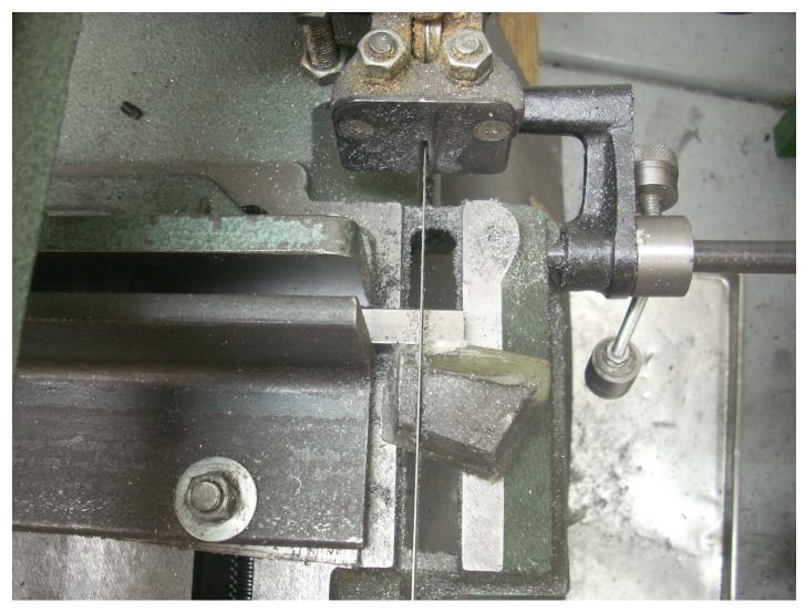
I started with 3 pieces of  $\frac{1}{2}$ " x  $\frac{1}{2}$ " x 12" CRS. All bars were cut about 0.05" longer than the finished dimension. Here I'm cutting one of the spacer blocks. My cutting "fluid" is a recycled block of paraffin wax. I collect the cut bits, melt them down in the sun, and cast them into a block again.
