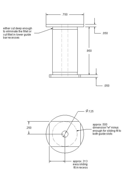
This should be the last part made. It is cut to fit the rest of the guide.
