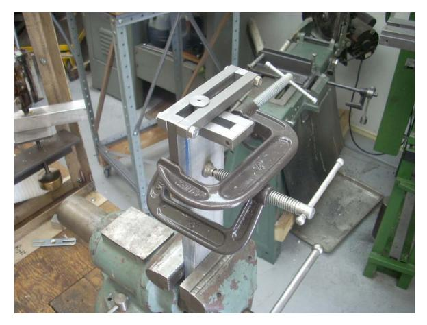
The drill guide has been clamped to a piece of 6061 bar stock held in my bench vise.
