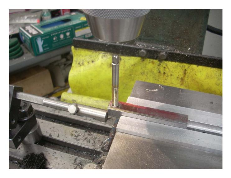
The spindle coasted to a stop and left the tap part way in the hole.
