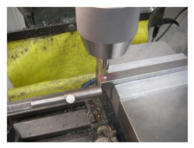
All bars *should* have been side milled on both ends but I only did one end. This worked well for the spacer blocks but could have been trouble for the horizontal guide bars.
