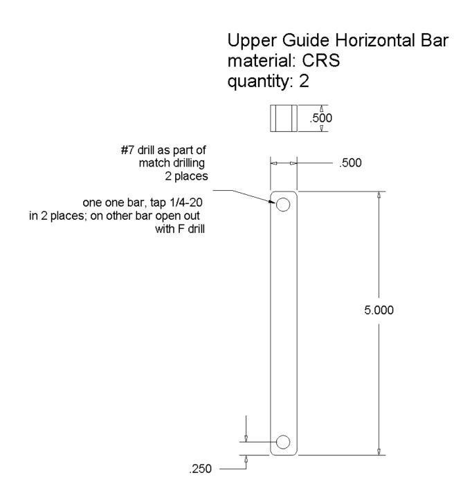
Neither of the 0.500" dimensions are critical. If you start with  $\frac{1}{2}$ " x  $\frac{1}{2}$ " CRS and take a light truing cut on all contact surfaces, you will end up with a thinner and narrower bar.
