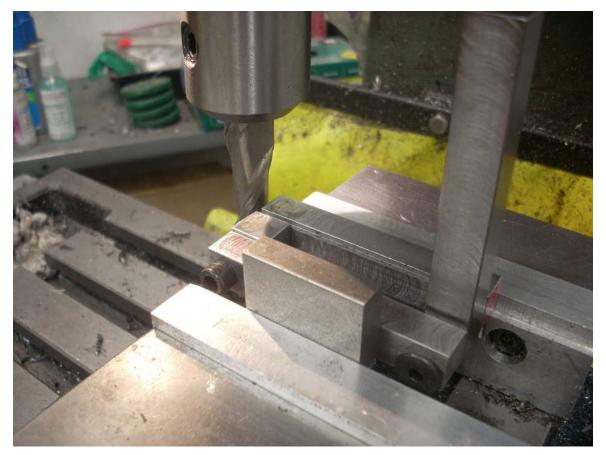
Here is why I thought I didn't want to side mill both ends of each bar. I figured I would assemble each guide and then mill it true on the end just for looks.
