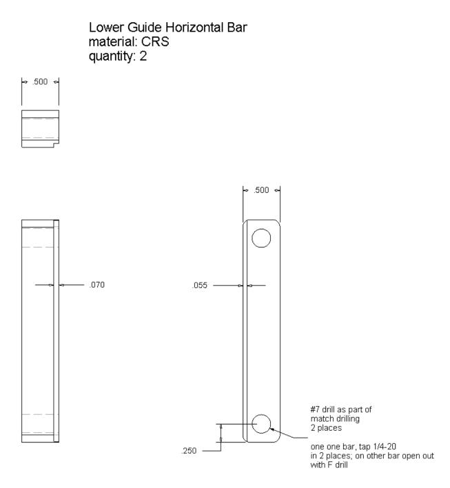
Neither of the 0.500" dimensions are critical. If you start with  $\frac{1}{2}$ " x  $\frac{1}{2}$ " CRS and take a light truing cut on all contact surfaces, you will end up with a thinner and narrower bar.
