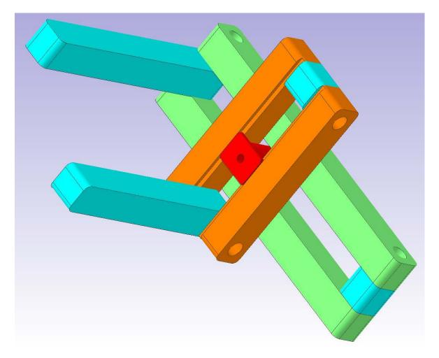
The underside of the guide reveals a bit more complexity. Shallow steps have been milled into the orange bars to accept a rectangular feature at the end of the bushing. This arrangement prevents the bushing from spinning as it guides the drill bit.
