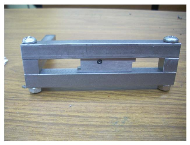
I used an expanding parallel to measure the space between guide bars. This assembly has the spacer block that was drilled correctly. The parallel slides nicely along the entire slot.
