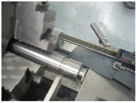
I then moved the parting tool over 0.950" + 3/16" in order to cut the underside of the second disk.
