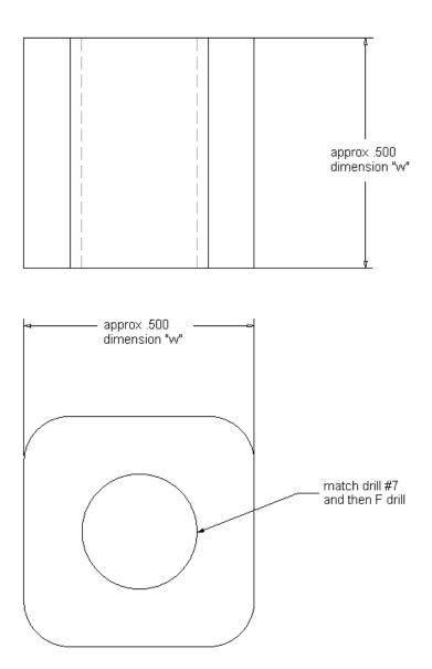
The thickness, "w", of these blocks must be identical to that of the vertical bars.
