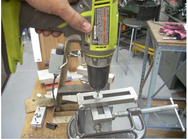
My drill press and mill/drill are too small to end drill a long rectangular piece of metal. It ends up in my vise where I try to use a hand drill and a lot of luck. This drill guide is my first attempt and finding a better way.
