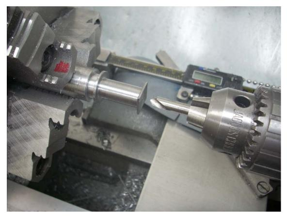
After feeding in to the finished diameter, "w", I moved the parting tool over by 0.050" + 3/16" and partially parted off the work piece. I then used my file to deburr the resulting disk.
