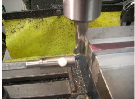
Time to side mill the ends of all bars. They were sawed fairly squarely so I can use a front face stop to position the end for milling. The stop is retracted and locked in position before the mill is powered up.
