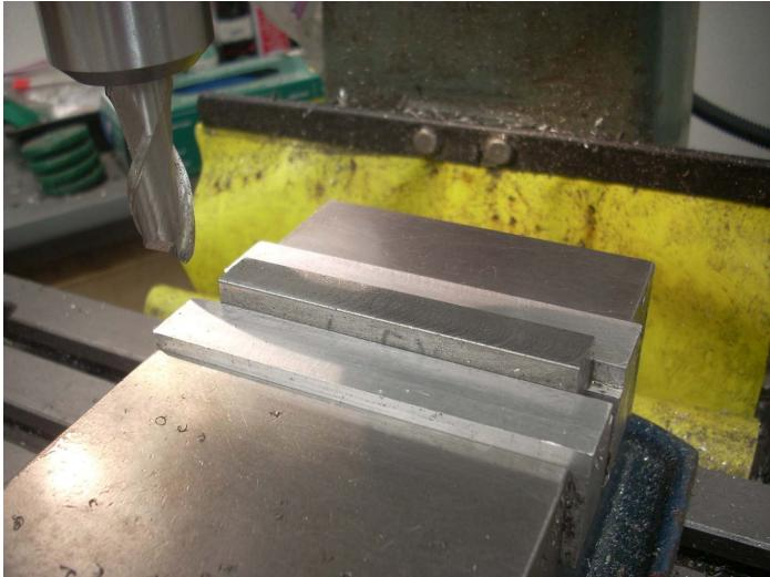
The vise is cleaned with alcohol and inspected to be sure no swarf is left on the contact surfaces of my soft jaws. I then pressed the first bar down and tightened the vise. The 5/8" end mill was then touched down on the surface, zeroed, moved to the left, and lowered about 0.004". The quill was then locked.
