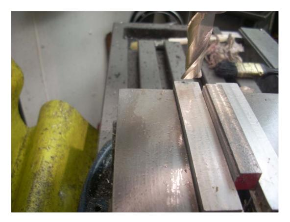
Here I'm milling in the steps into the lower horizontal guide bars. Once the cutter's position had been locked, I milled one bar, carefully cleaned the vise with alcohol, and then milled the second bar.
