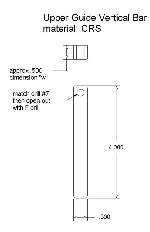
The thickness, "w", of this bar must be identical to that of the other vertical bar and of the two spacer blocks.
