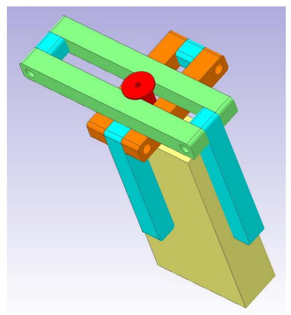
The accuracy of this guide depends on having a close sliding fit between the two slots and the bushing. The trick is to machine the width of all blue bars at the same time. The actual thickness is not important, just that they are all the same. After assembly, the width of the slots are measured and used to define the diameter of the bushing.
