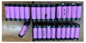
At this point, my ambitions were reduced to collecting individual LiPo cells. I desolded the groups and performed a final voltage check. All still read 4.1 volts. A load test might expose
