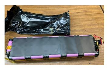
Peeling off this film, I found rigid plastic sheets further protecting the cells. At this point, I discovered that Lectric had used Samsung 18650 29J cells.
