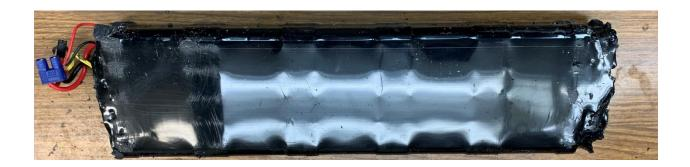
The output terminals and switch were connectorized, so I removed them. The cells and Battery Management System were wrapped in a heavy black plastic film.
