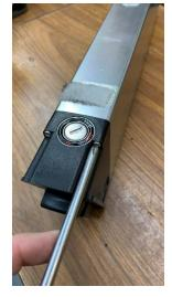
There are three easily accessible screws on each end of the battery. Oh boy, this is going to be easy.
