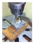
Next up is the tapping of the bottom plate. I could use the tap drill to set alignment but the tap works fine. The drill press is brought up to speed, then power is cut as I drive the tap into the tap hole.
