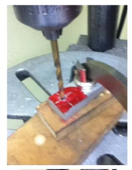
I now recut the top plate with a clearance and counterbore hole. The first step is to align the hole with the center of rotation of the drill chuck. I do this by reinstalling my tap drill and feeding it into the hole. Then I clamp down on the part. I have added a second piece of MDF to raise it up a little because I have limited depth range on my drill press.
