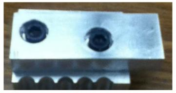
Once deburred, I installed both screws which have to be a perfect fit due to the method used.
