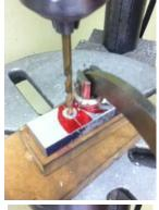
I then separated and deburred the two part. After mounting the tap drill again, I use it to align the top part.
