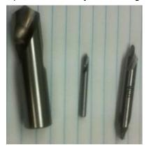
best tool for cutting my starter cone. A center drill is really design to cut a cone in stock to be mounted on a lathe. A spotting drill is the proper tool. I have to admit that I did know better but could not find the proper size.
