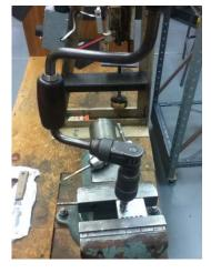
After the tap has been removed, I used a countersink mounted in a brace and bit to deburr the hole. One or two turns does the trick and leaves a very smooth little chamfer.
