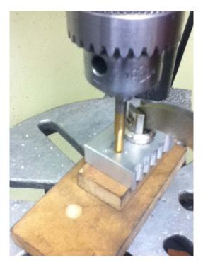
This next step takes a lot of care to do right. I chuck up my spiral tap and position it above the hole. Power is applied and I wait for full speed to be reached. Then I cut power and plunge the tap into the hole.
