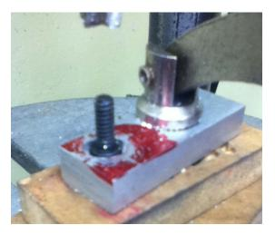
I am using the screw's head to gage the depth of the counterbore hole. This is done with the machine off. The end mill removes fingers far better than it removes metal.
