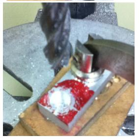
Then I switch to my end mill to cut the counterbore hole.
