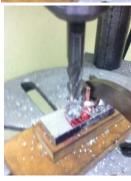
And finally, I use the end mill to cut the counterbore hole. I then remove the part and deburr it.
