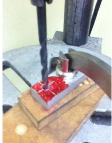
With the part aligned on the tap drill, I switch to my clearance drill and go all the way through this top piece.
