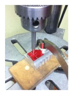
Using layout fluid, I have marked the location of my first screw. Note that both pieces of metal are clamped into position. My spud helps me set the center of rotation of the drill accurately on the cross lines. The stack of metal rests on a piece of scrap Medium Density Fiberboard (MDF) to protect my table.
