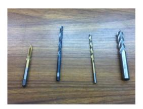
Here are the tools I will use. On the far left is a 3 flute tap. It will cut a 10-24 thread. The "10" refers to the diameter of the screw that will fit this hole and the "24" is the number of threads per inch.
