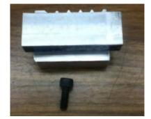
I will use what are called Socket Head Cap Screws (SHCS). You can barely make one out at the bottom of this picture. The screw has a hexagonal hole in the top to drive it with an Allen Key.
