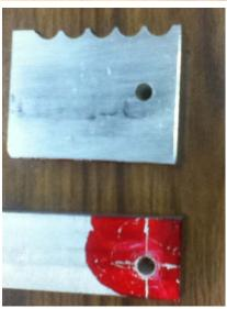
I then used my tap drill and went through both pieces at the same time. This is what match drilling is all about. The resulting hole must perfectly align in both pieces because they were cut in the same pass. The parts have been unclamped because the remaining steps are done separately on each part. Before proceeding, I deburred both holes.
