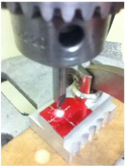
I am using a centering drill to make a small cone shaped hole in the metal. This tool has a small cutting diameter but a large body diameter. There is much less tendency for deflection of the drill with this tool. If I used a small diameter drill, it is likely it would bend as I started the hole and when it finally did start to cut, would not be at the cross lines.
