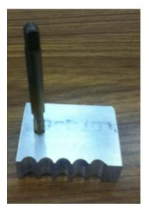
Terrible picture but I hope you can make out that the tap is stuck in the hole. I will use a tap handle to turn it all the way in and then remove it.
