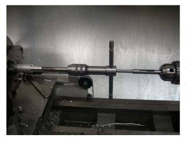
I then center drilled, followed with a Q drill to a depth of 0.6", and ran through with a 3/8 - 24 tap.
