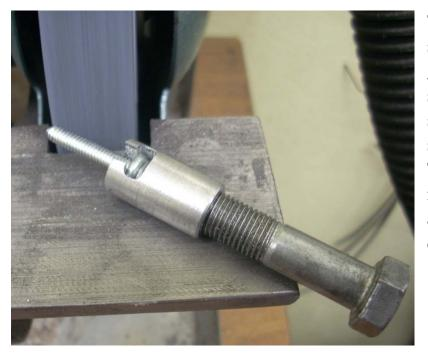
This vise clamps screws for safer handling during grinding. To clamp the screw, back out the bolt, slide the screw into the side slot, and tighten the bolt. The smooth, round body makes it easy to turn the vise and grind a bevel on the end of the screw.
