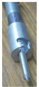
Here is the finished vise with a #8 screw in place. The 3/8 - 24 bolt that makes up the handle has a slight cup in the end which helps to align and hold the screw head.
