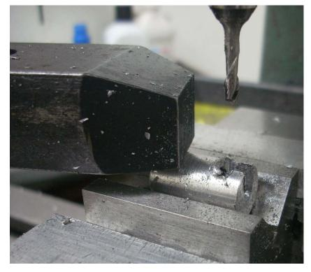
I milled the side slot using the same end mill.
