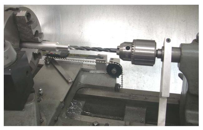
My first step was to turn down some 5/8" diameter aluminum rod to an OD of 0.500".
