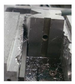
Here is a side view after the end slot was cut. Because of the small diameter of my end mill, I took a series of light cuts and hand fed the motion. It is all too easy to snap off such a thin end mill.
