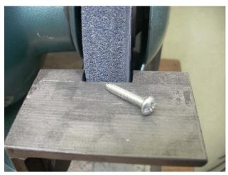
Previously I was faced with trying to hold the screw with pliers and then smoothly turn it to grind a bevel. Using my fingers may have given me better control but one slip and I could be hurt.
