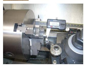
I used my caliper to determine how much more metal to remove and then trimmed to the final length.
