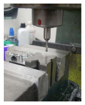
I used a V block to help clamp the part with the small hole end facing up. My 0.1" diameter end mill was centered in the hole by eye and my Digital Read Out zeroed in the X and Y direction. I lowered the end mill until it touched the part and zeroed the Z axis.
