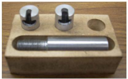
The second improvement was to mill a block of 5/8" thick MDF to hold my new tool. I plan to make one more head so left a hole for it. This head may be for #4 screws or for #10 screws. If I decide to make a #4 holder, I will forgo the side slot and just have a center
