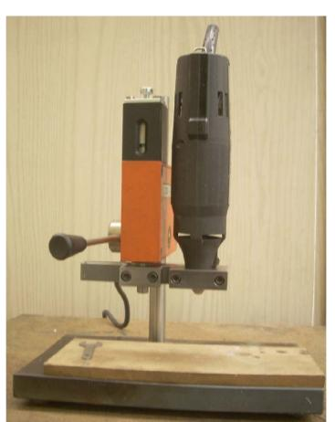
I replaced that broken top with a piece of aluminum. The holes were match drilled through the black rectangle below it so no measurements were needed. I discovered that the hole in the center of this top had a brass threaded insert so I drilled and tapped a similar hole in my new top. I discovered that by adding a screw I was able to adjust the spring tension.
