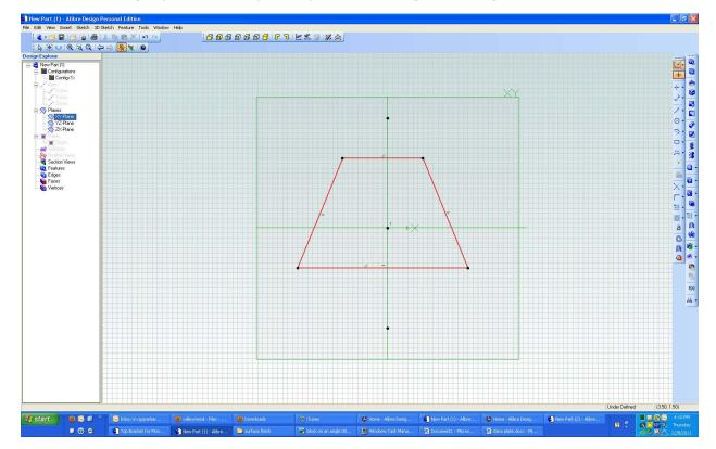
I start with my XY plane selected and draw a reference line vertically through the origin. The plate is symmetric about this line and I will call this my Line Of Symmetry (LOS). Then I drew my outline. It is not constrained to be symmetric yet.
