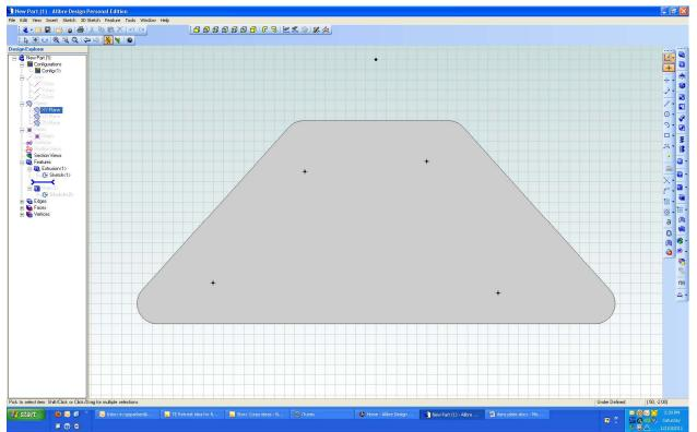
I now get the outline of the part plus 5 nodes. The top node which is off the part is my origin. The four nodes on the part are the centers of all holes.
