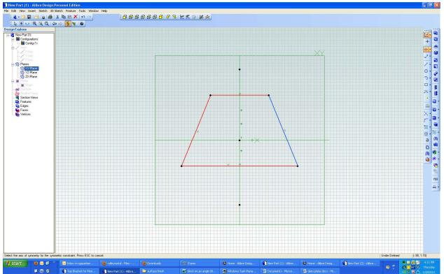
Next I selected the symmetric constraint tool and clicked first on my LOS. Then I clicked on the two sloped lines which now snap into being mirror image.
