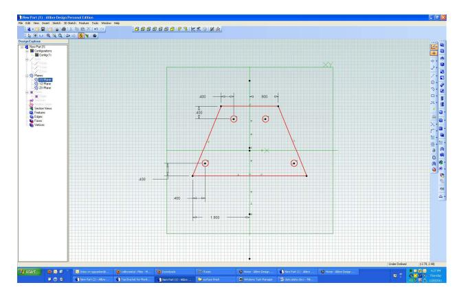
I placed my left two circles in their exact position relative to the corners of the part. Then I used the horizontal constraint to force the bottom right circle to be at the same height as the bottom left circle. The same was done with the upper two circles.
