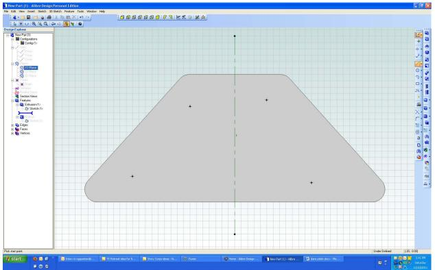
The first thing I want to do is draw a reference line from the origin and down across the part. This will enable me to place my holes in a symmetric pattern.
