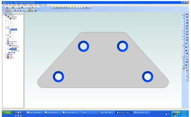
Exiting the 2D edit mode, I now have my 3D plate with four countersunk holes in it. I liked the look of it but exact dimensions have not been applied so this is not yet usable.
