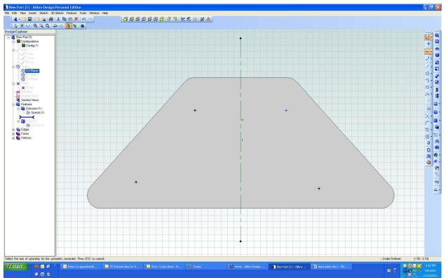
As with the outline of the part, I again used my symmetric constraint tool to force the top two hole centers to be mirror images. I click on the LOS and then the two top centers. Since I clicked the left center first, the right center moved to be symmetric with it after I clicked it.
