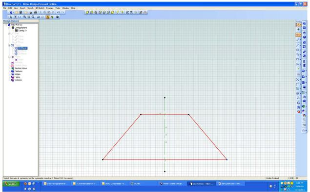
Using the symmetry constraint tool, I defined the top two corners to be symmetric by first clicking my Line of Symmetry (LOS). Then I clicked the upper left corner and the upper right corner. Moving either of these corners will move the other one. I did the same thing with the lower left and right corners: click the LOS followed by clicking each of these two lower corners.
