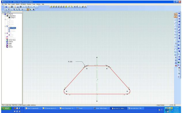
Without putting the radius tool away, I applied the same radius to the other three corners. Note that each one has an "=" sign next to it. This means that changing the one that is dimensioned, I will change all of the corners by the same amount.
