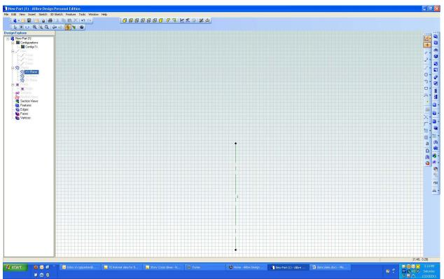
After opening a new window and selected the XY plane, I drew a reference line from the origin down to around 3".
