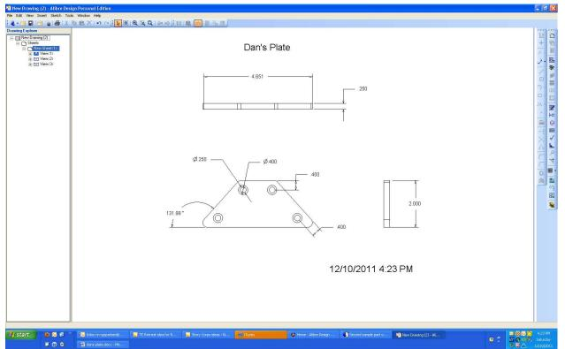
My final touch was to go to the menu, select Insert and then annotation. Then select Note. The Note tool was then used to label the part and add the date and time.
