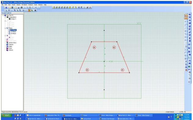
I have roughly placed the four holes. Since all holes are the same size, I drew my first hole, and then when I drew the rest, I adjusted the size until I saw an "=" sign. Their diameters are then locked to be the same.
