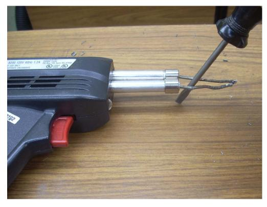
You could buy a purpose built demagnetizer but an old soldering gun works well.
