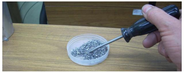
Here I have a dish of steel swarf and a low cost screwdriver. I dipped the screwdriver into the swarf.
