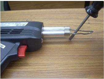
I then turned on my soldering gun and passed the tip of the screwdriver through the loop as shown. The gun produces a magnetic field that reverses direction 60 times per second so returns the screwdriver to its non-magnetic state with the magnetic domains facing in random directions.
