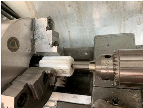
Going to my lathe, I first cut a bevel in each end. Then I drilled a 1/4 inch hole in each end to a depth of 0.9 inches. This was necessary to meet the required overall length.
