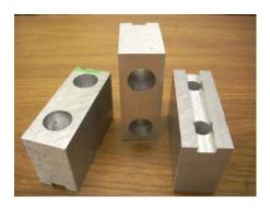
This setup is ideal for installing soft jaws. I don't believe I need such a precision fit, just need to clear the major features. I have just knocked clearance holes with counterbores in blocks of aluminum. The milled slot is a very loose fit. These will not be as solid as the hardened jaws but then I don't intend to hog a lot of metal either.
