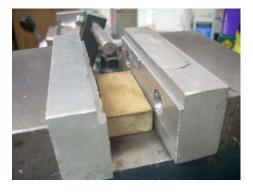
The problem is easily solved by placing a piece of 1/2" Medium Density Fiberboard (MDF) down on the vise ways. MDF is remarkably uniform material with the top and bottom faces parallel within a few thousandths of an inch.
