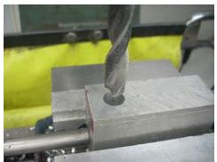
Starting with a  $\frac{1}{4}$ " drill, I go all the way throughout the block and into the MDF. In order to prevent chips from clogging around the end of the drill, I drill only about  $\frac{1}{4}$ " before bringing the drill up. I then follow with my clearance drill.
