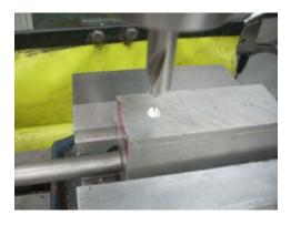
I watch my DRO to guide me to the first hole. Then I run a spotting drill to cut a small cone shaped hole.
