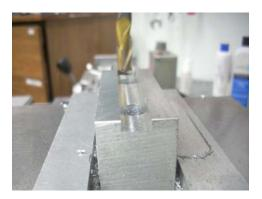
After all holes were drilled, I swapped out my drill chuck for my 1/4" end mill. I then cut a slot in the bottom of each block.
