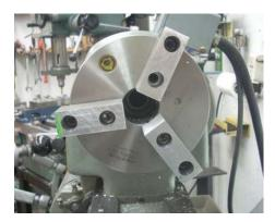
Here are my soft jaws installed on my chuck. There is plenty of metal available to shape into any fixture when the need arises. Then it can be re-cut for the next fixture.
