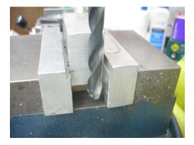
I first take out the cutting tools I plan to use to be sure they can all reach. My longest tool is my 5/8" drill. The shortest tool is my 1/4" end mill. I want to set the height of the mill head so I can do all operations without moving the head. Any such movement will cause me to lose XY position.
