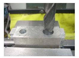
With all 3 blocks drilled with clearance holes, I chuck up my 5/8" drill in order to cut my counterbore. I may later cut the bottom flat but must make a cutter for that first.
