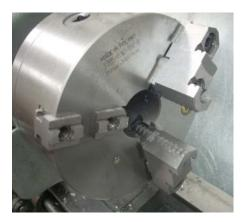
My Bison lathe chuck has served me well for many years. One of its features is the ability to remove the jaws from sliding supports and point them in the opposite direction. This is handy when I want to hold a part from the inside.
