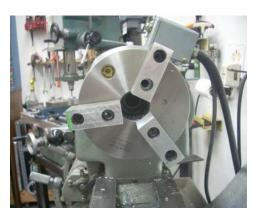
Here are the soft jaws almost completely installed. One screw is left to install.
