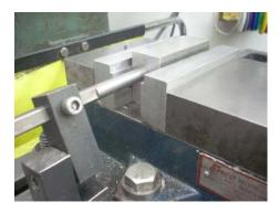
I started by selecting some 6061 aluminum that roughly approximated the hardened jaws outer dimensions. Blocks were then cut on my bandsaw, deburred, and cleaned. I then set up a stop on my vise so each block will be in the same position. I then realized that this won't work because I need to drill through holes. I would end up drilling into my vise ways.
