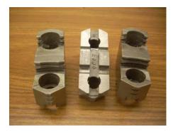
The jaws all have unique numbers and are a precision fit on their bases. They feel like they were lapped into place. I'm sure this provides a great deal of strength since surfaces exist in this interface to prevent any lateral motion.
