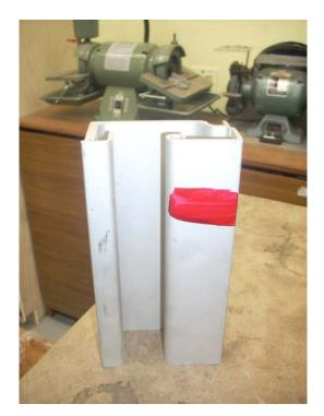
This next approach has the advantage of not needing access to the chuck or the tail stock. I pulled a piece of extrusion from my junk pile. It will sit on my lathe ways which are flat. At approximately the height of the centerline, I have put on a stripe of layout dye.
