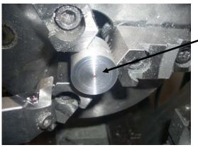
After making a pass with my cutter, I was left with this nub. Only a close inspection tells me if the cutter is too high or too low. When set exactly on the height of the center of rotation, there will be no nub.
