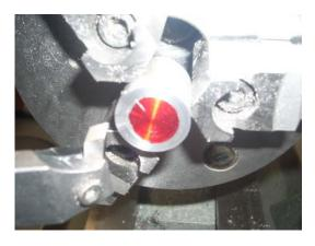
Regardless of the method, it is good to test the result until you are confident. The best way I know to verify tool height is to take a test cut on a scrap of aluminum.
