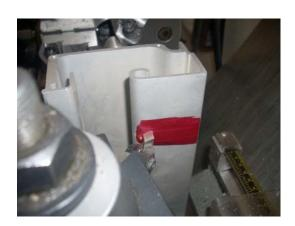
I then take my cutter which has already been set exactly on the center line, and press it against the extrusion.
