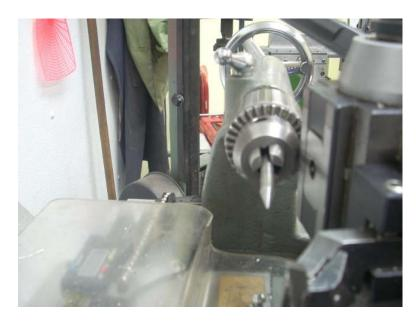
Another way to set the cutter at the center line is to chuck a "spud" into the tail stock.
