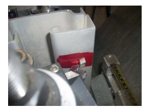
Then I run the cross slide in, causing a line to be scribed. I now have a cutter height tool that can tell me when my cutter is at the lathe's center of rotation height.
