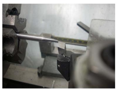
In that case, you may be able to chuck the spud into the head stock's chuck.
