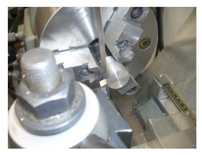
Maybe the most elegant and popular way to set a cutter is to use a small steel ruler. Simply pin the ruler between a piece of round stock and the cutter. When the ruler sits vertically, the cutter is right on the center line.
