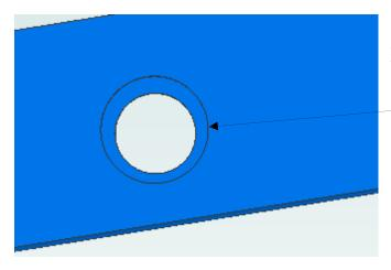
The tube that will accept the male part of the fastener is first drilled 3/8" through. Then the outer face is drilled 1/2".
