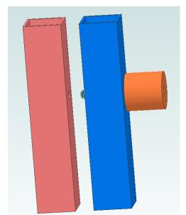
I needed to be able to fasten two pieces of 16 gage 1" steel tubing together. There shall be no loose parts and no tools required. A misalignment of  $\pm 1/16$ " shall be tolerated. The fastener thread is  $\frac{1}{4}$ -20 and 4 to 5 threads shall engage.
