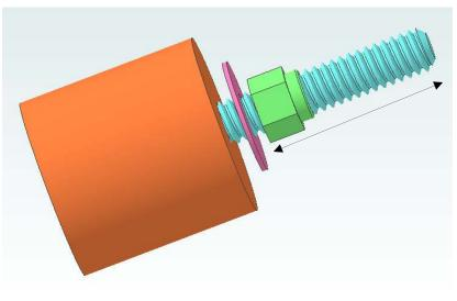
The male part of the fastener consists of the knob, a washer, a self locking nut, and the threaded rod. The ends of the rod are generously beveled.
