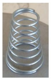
I bought this spring at Ace Hardware. The small end has an ID of about 3/8" and the large end has an OD of about 3/4". The overall length is about 1" uncompressed.
