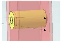
This arrangement solves two problems. The threaded material is ample compared to just trying to thread the wall of the tubing.
