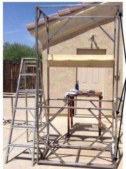
The fasteners are part of a structure that is occasionally set up in various places and then knocked down into 4 flats for transport and storage. It is 2' deep, 4' wide, and 8' tall.
