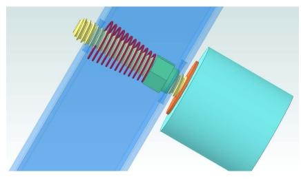
I was contacted by Bill Libecap on an idea that employed a spring to retract the fastener plus keep it from flopping around when disengaged. After a bit of discussion, we came up with this modification to the design. A conical spring has been added.
