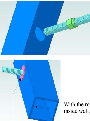
The rod/nut assembly is then fed into the tubing through the  $\frac{1}{2}$ " hole. Note that the bottom of the nut is towards the tubing.
