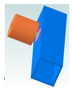
The aluminum knob goes on next but this is a thermal fit. The hole in the knob is first heated with a  $MAPP^{\text{(B)}}$  gas torch for 20 seconds before being tightly screwed into place.
