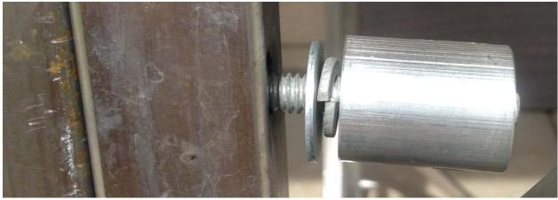
I have added a spring washer between the knob and the regular washer for this application. The knob was intentionally left smooth because very little force is required. Compression of the spring washer is all we need.
