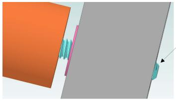
This distance lets the beveled end of the rod barely extend beyond the face of the tube. There is enough exposed to help with alignment but not enough to be snagged during transport.
