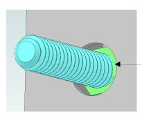
The  $\frac{1}{4}$ " diameter threaded rod passes through the  $\frac{3}{8}$ " hole to give  $\pm \frac{1}{16}$ " of free movement.
