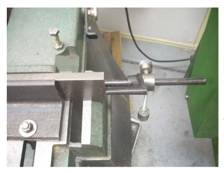
The whole point of having a stop is to provide a repeatable reference surface. But on a saw, there is another essential feature - the stop must be removed before cutting. Otherwise, the severed work piece can jam between the blade and the stop at the end of the sawing process. The original stop lost its position when rotated out of the way.
