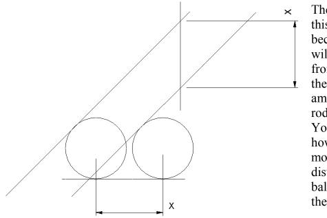
The reason I think this works is because the balls will all move out from the center of the gage the same amount as the push rod moves down. You can see here how the 45° line moves down a distance "x" and the ball moves over by the same distance.
