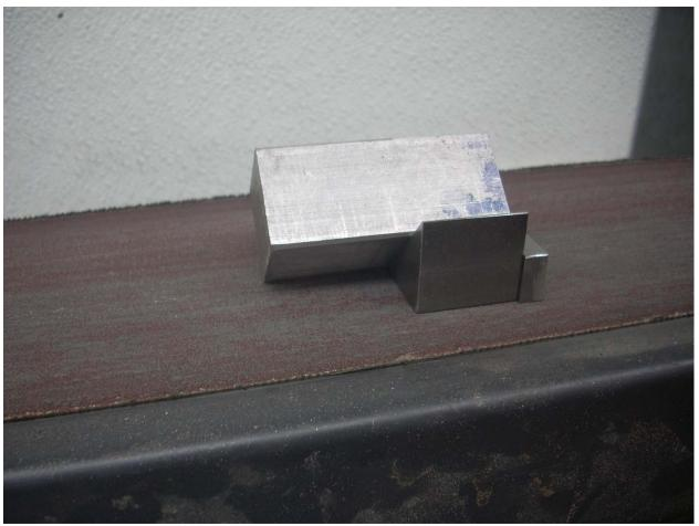
With the belt moving, I placed the block of aluminum in the fixture and lowered the assembly down. The belt made short work of the corner and give a uniform bevel.
