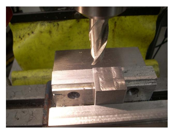
The side milled end is now down on my softjaws and I end milled the top face to an overall height of 1". The dimensions are not critical but the block should be square.
