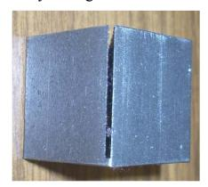
I removed the block with about 0.1" left to cut. The top of the kerf had bent in and I used a screwdriver to pry it open again.
