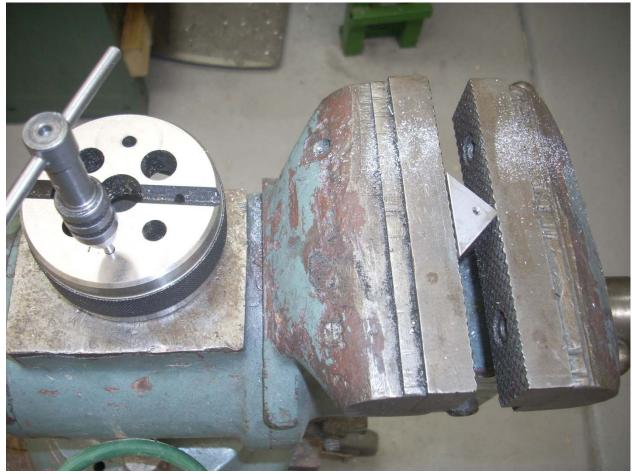
I used a bench block and a 6-32 spiral tap to thread my first hole in the wedge. The pilot hole was drilled extra deep to accept the swarf given off in the tapping process. Hand taps eject swart out of the hole while spiral taps push it down in the hole. However, a sharp spiral tap lets me feed down the hole without backing out to break the swarf which is very nice.
