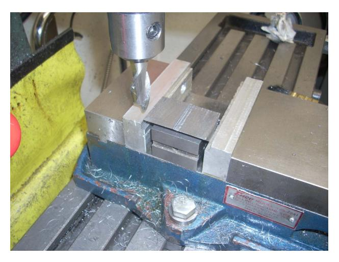
I placed the two wedges in my V block and clamped it in my mill vise. The clamping surface is smaller than I like so I took light cuts.
