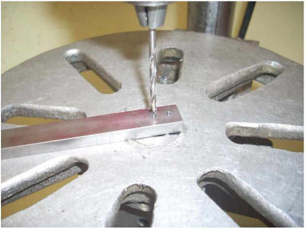
Using the tap drill for a 6-32 screw, I knocked two holes in the support bar on my Gingery drill press.
