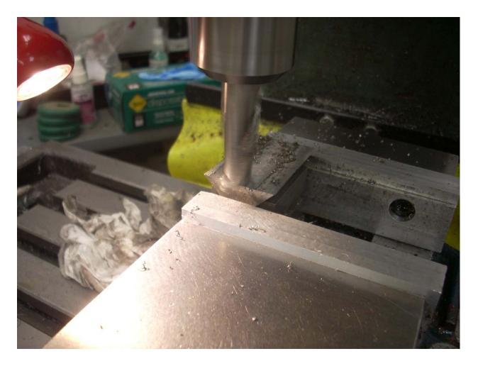
I chose to take my first light cut down the center of the part. I am removing the most material but the forces are balanced so the risk of having the wedges tilt is minimized. Subsequent cuts were narrower and more likely to cause tipping.
