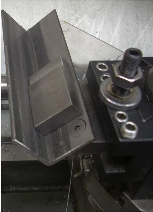
To bevel a block of metal, just slide the edge along the bottom of the channel with the lathe running at the proper speed for this diameter end mill. It might take a few passes to get the edge cleaned up nicely.
