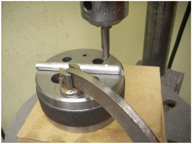
I can then change to a different drill and be confident that the hole I cut will be on the center line of the round stock. I'm using a spotting drill here to cut a cone shaped hole.
