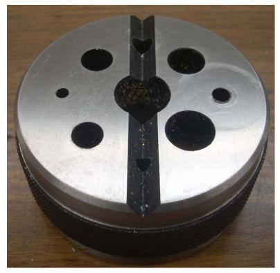
The top surface has been ground flat with respect to the bottom. Use it when you need to raise something up while keeping it parallel to the support surface.
