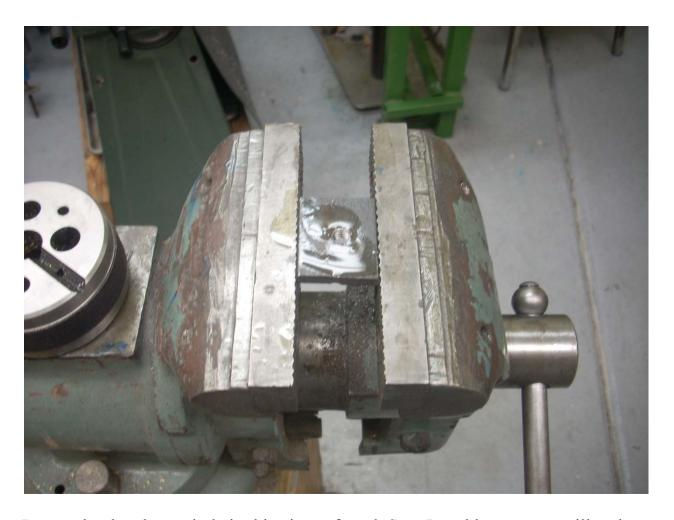
I wanted to hand tap a hole in this piece of steel. Sure I could set up my mill and install my tapping head, but it is hardly worth the trouble. The tap must go in reasonably straight but I didn't need super precision here. So I put the steel into my vise jaws so it was aligned with the top of the vise jaws.
