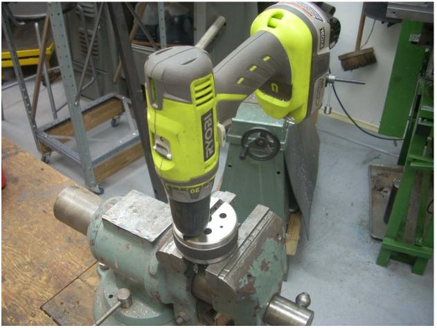
There are plenty of times that I want to drill a hole using my hand held drill. The block provides a degree of alignment that I have trouble reaching by eye.
