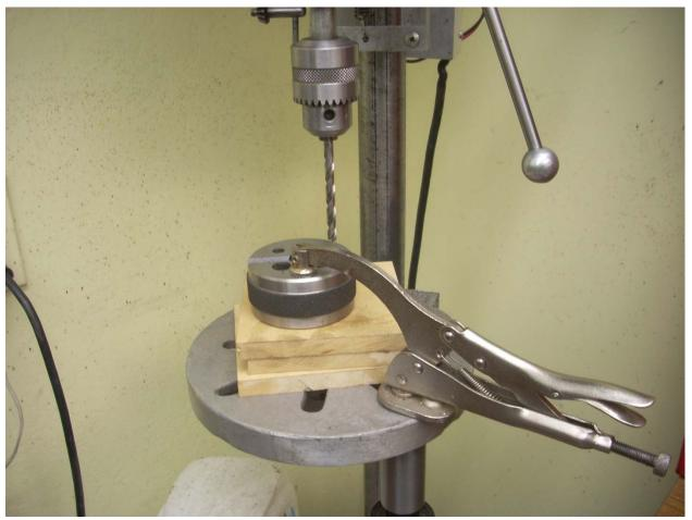
The bench block is also useful on my drill press. Here I have installed a ¼" drill in the chuck. Then I fed down until the drill entered the ¼" hole in the V.
