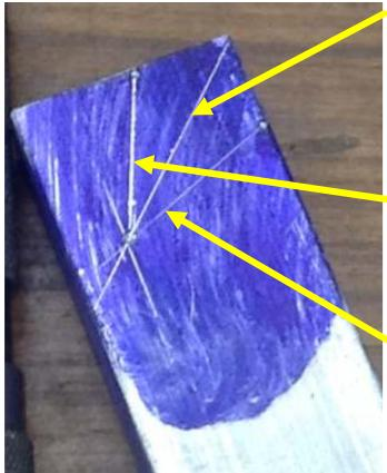
Using the square's  $45^{\circ}$  end, draw a line from a corner to the far side of the workpiece. Then scribe a line  $\frac{1}{4}$ " from that far side that intersects the diagonal line. Use the punch to mark this point. It will be the bottom of the V.
