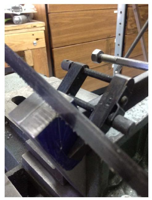
The two work pieces were placed in the band saw's vise such that the first line could be cut. The punch marks were facing the pivot of the saw.
