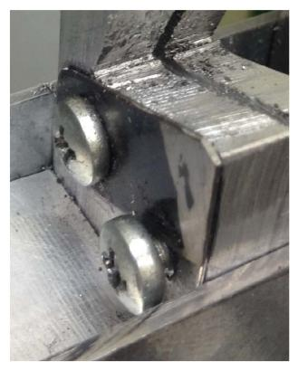
I used a tap, so ran a #36 drill in to form a hole that flanked the bottom edge of the hacksaw blade. The idea is to prevent the blade from sliding away from the bolt resting in the V. Note that this second bolt was not tightened all the way into the thread plate. When I did that, it pushed the hacksaw blade up. As shown, the hacksaw blade is solidly mounted.
