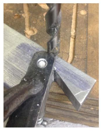
Selected a drill bit who's end snuggly fits through the hole in the hacksaw blade. Drill in enough to form a small cone.
