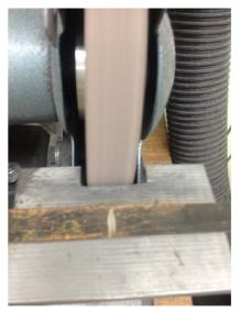
I didn't need the entire length so used my grinding wheel to score both faces about 2" from the end. I did preserve the rounded end and mounting hole. It then easily snaps off.
