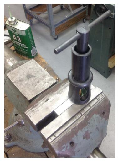
The block went into my vise with the side were flush with the top of the jaws. I then squirted a little cutting fluid into the hole to make tapping easier.
