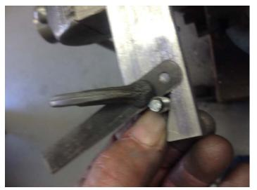
I could have used a lot of math to figure out exactly where to place the thread plate. But the direct method is far less work. I took a <sup>1</sup>/<sub>4</sub>-20 bolt and place it in the V. Then the beveled edge of the hacksaw blade was pressed into the threads so the bolt could not slide in and out. The clamp was then loosely tighten to the hacksaw blade.
