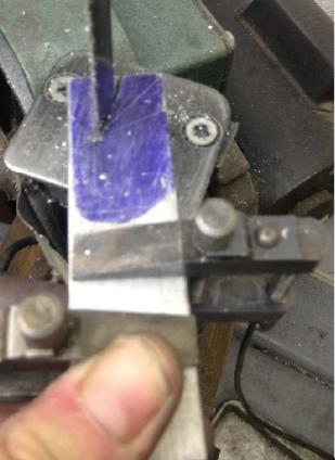
The work pieces were removed from the saw's vise and I freehand cut to the punch mark.
