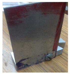
The clamp was then removed and I ran a bolt through the side plate and into the threaded hole in the block. With the end of the block resting on the table and the plate's bottom edge also resting on the table, I tightened the screw. This insures proper alignment of the plate and block on the bottom.
