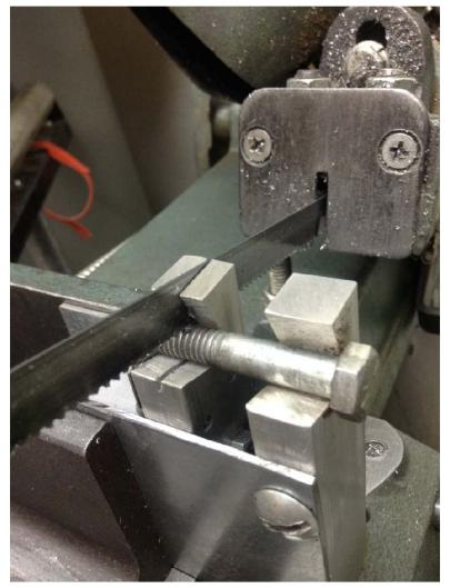
This fixture evolved from a previous design that only handled <sup>1</sup>/<sub>4</sub>-20 bolts. It can now handle bolts <sup>1</sup>/<sub>2</sub>" in diameter and smaller both in metric and English. It also references the underside of the head to set overall length.
