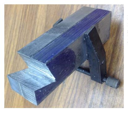
I then had two work pieces with identical V cuts in them. You could smooth the surfaces with a file if you like but take care not to open out the bottom of the V.
