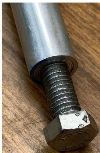
With the anchor locked into the tubing, I screwed in my 3/8-16 bolt.
