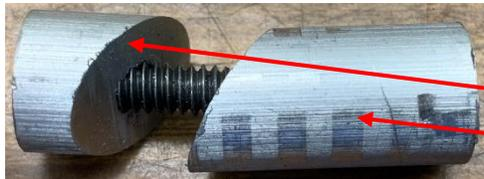
As the SHCS is tightened, the lock is drawn into the body. The angled faces cause them to shift out
