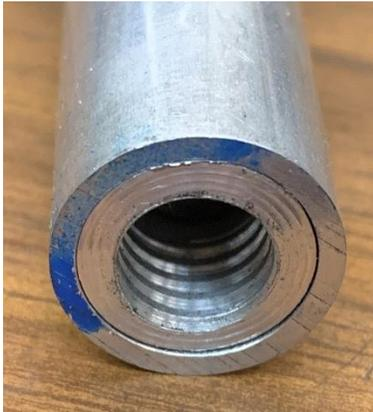
Here is one example. I have thin-walled aluminum tubing with an inside diameter of 1/2". I want to screw in a 3/8-16 bolt. My homemade anchor solves the problem.
