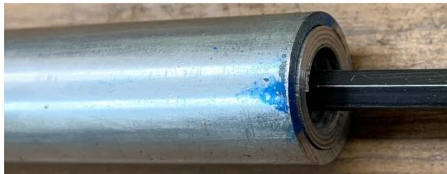
I have found that the lock digs in well enough that I do not need to grab the body as I tighten the SHCS. This lets me set the anchor flush with the end of the tubing.
