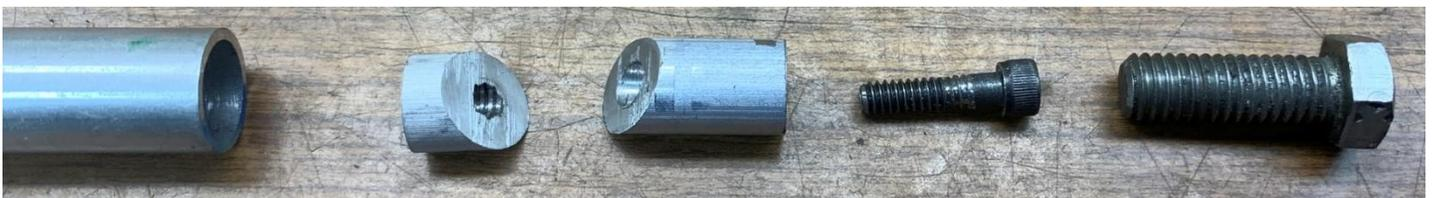
Here is the finished anchor laid out in pieces. The smaller screw feeds through the larger cylinder and into the smaller cylinder. As it is tightened, the smaller cylinder moves sideways and locks the assembly to the inside of the tube. Then the larger screw threads into the top of the larger cylinder.
