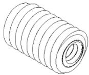
One option is to drill and tap a short length of 3/8-16 rod to accept a 10-24 thread. Then I would screw in the rod coated with Loctite Red. This would give me my smaller threaded hole. But there is problem with making it permanent. I cannot feed a hex wrench down the hole to unscrew the SHCS. If I went with a 1/4-20 hole in the 3/8-16 rod, my hex wrench could pass but now I'm back to an over-sized screw.
