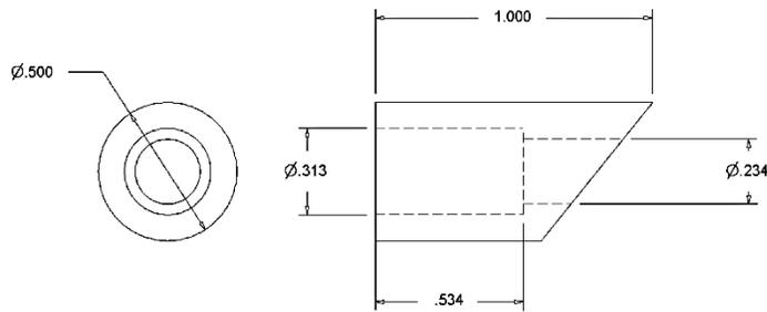
0.313” hole, it would not have been possible to make the hole small enough to accept a 10-24 tap. Hence, I accepted the 3/8-16.
