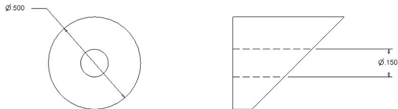
The lock is made from the same material as the body. After drilling the hole, tap it 10-24.
