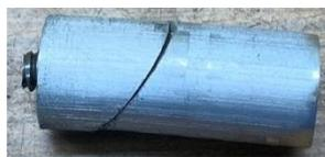
of alignment. Since they are both a close sliding fit to the bore, this shift causes the lock to dig into the wall of the bore.
