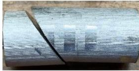
sawing the end of the part off. Just be sure you cut at the threaded end. File the cut faces smooth and you are done.
