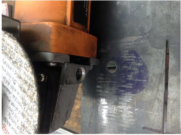
We must next locate the hole for mounting the plate to the grinder. On my grinder, the handle hole was threaded 3/8-16. I took a piece of threaded rod and turned a point on it with my lathe. If you don't have a lathe, just skip the point. File the end of the rod flat. Then roughly locate where the hole will go on the plate and blue the surface. Don't have any bluing? Use marker.
