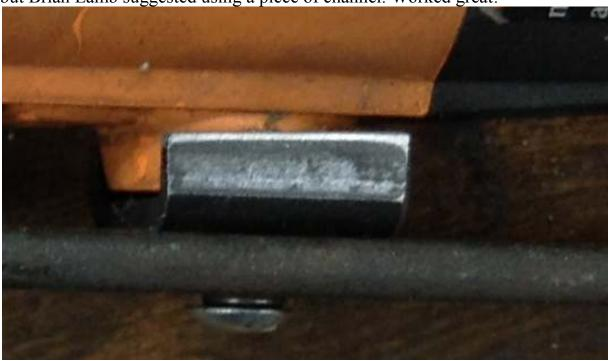
I through drilled the bar and drilled and tapped 10-24 into the channel.
