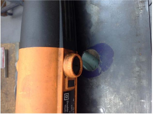
Use a pencil to roughly mark the location of the motor brush boss. Then use bluing or marker to paint the area. Finger snug down the grinder to the plate and scribe around the boss.
