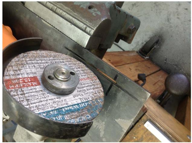
Clamp the plate into a large vise or over the edge of your work bench. Draw a line with a marker about ½" from the side edge and about 1" from the end. Then, holding the abrasive wheel as close to parallel to the edge as possible, carefully plunge cut through the plate.
