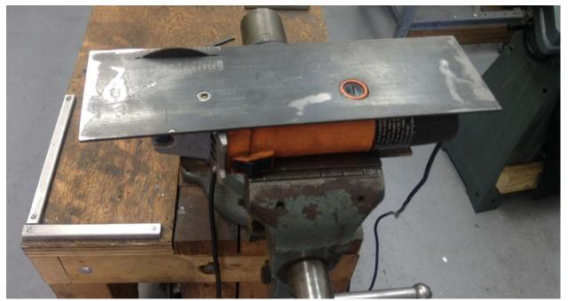
With the lower bar clamped into my vise, I have a solid work table for abrasively grinding heavy gage sheet metal into small pieces.
