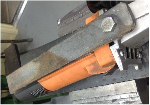
With the bar bolted to the lower handle hole, I have a solid place to clamp the assembly with my vise.
