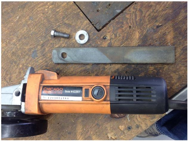
I then raided my scrap pile for a piece of steel bar ¼" thick, 1" wide, and about 7" long. It happened to have a hole in one end so all I needed to do was use it. I also found a ¼" thick homemade aluminum washer to raise the bar so it was roughly even with the top of the lower motor brush boss.
