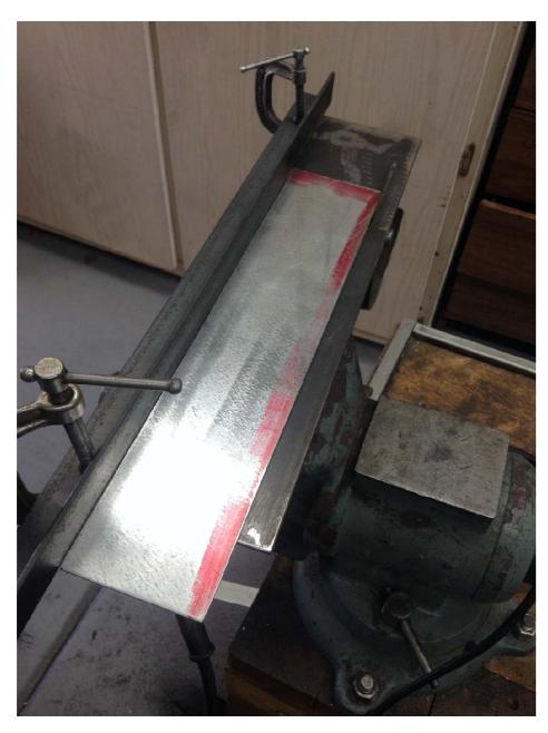
I needed to cut 10 gage steel into a strip 2.5" wide.
