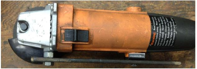
After the article was published, John Herrmann suggested that I capture the lower boss in the support bar to prevent the grinder from pivoting. The bar is too narrow but Drien I amb suggested using a piece of sharped. Worked great!
