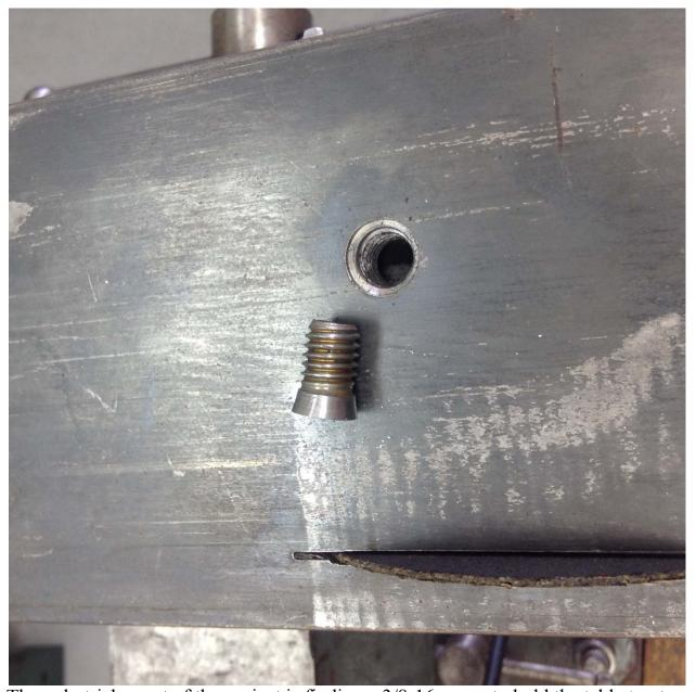
The only tricky part of the project is finding a 3/8-16 screw to hold the table top to the top handle threaded hole. Since I have a lathe, I took a button head screw and reshaped the head. If I happened to have a flat head screw in my junk drawer, I would have used that instead. The goal is to get the top of the screw flush with the top of the table. If necessary, you can counter sink through the plate and also into the aluminum head of the angle grinder.
