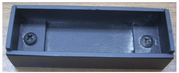
The screw on the right is 6-32. The screw on the left was supposed to be 6-32 too but I accidently ran my clearance drill through the channel. The easiest recovery was to go up to an 8-32. After the screws were set, I placed the box on my belt sander and made them flush.
