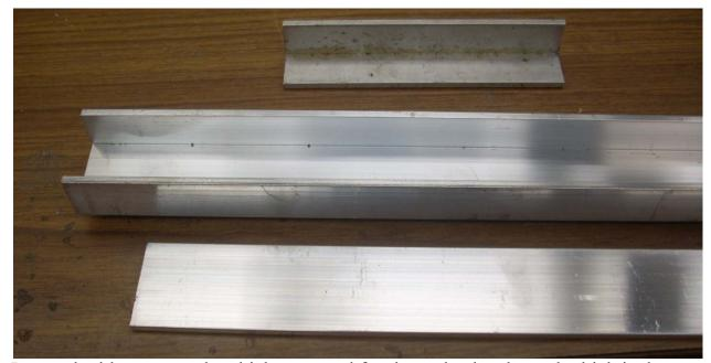
I started with some angle which was used for the ends, the channel which is the body, and the plate which is the top.
