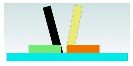
When we flip around the black blade and put it up against the yellow blade, there is a gap. The angle formed by these two blades is twice the difference between the blade angle and true vertical. We move both blades roughtly the same
