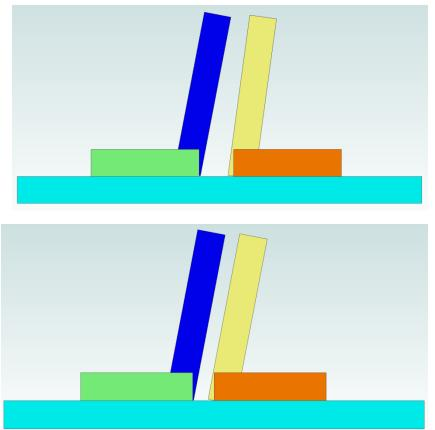
The yellow blade square we wish to set true is put up against a blue blade square of unknown accuracy. In this exaggerated view, they are both off in the same direction but neither is near true.
