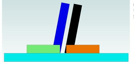
and adjust the black blade to match the angle of the blue blade.
