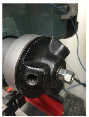
Paul Thompson noticed there was a flaw in my plan. Not only must the quill be set to Home, the gear train from drive motor to pinion gear must not change relative position. Variation in these gears contribute to error.
