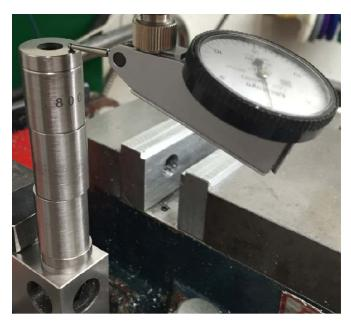
10. You are finally ready to actually input data. At the moment, I am at Home. My DTI is resting on top of my stack of spacer. The DTI has been zeroed and both the Machine Coordinates and my Z DRO read zero.
