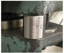
I raise up my quill until this 0.7000 inch tall spacer block does not fit in this gap. Then I lower the quill 0.0001 inches per step until it just slides in place. The quill is then at Home. By lowering the quill until I reach Home, backlash is avoided. All subsequent measurements were taken by lowering the quill down on spacer blocks.
