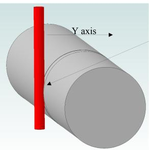
Remove the end mill<sup>2</sup> and install a length of drill rod of known radius. Position the rod such that its side just contacts the cut surface.
