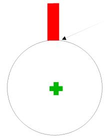
Here is an end view of just the cut surface. The bottom of the end mill is tangent to the surface. It doesn't matter if the end mill is *exactly* aligned with the COR. The further off alignment, the more cupped will be the cut surface. You may need to move the spinning cutter along the X axis in order to form a flat surface. We need this flat surface in order to accurately measure the diameter.
