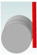
As a check, move the rod to the opposite side of the workpiece and verify you read the sum of the radii.
