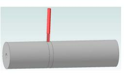
Check the Z axis zero by moving to Y = 0 and take a skim cut. Verify that your Z value equals the radius just cut.
