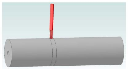
I mounted my stock in the A axis drive and installed a ¼ inch 3 flute end mill in the spindle. By eye, I centered the cutter at the Center of Rotation (COR) along the Y axis and took a skim cut.
