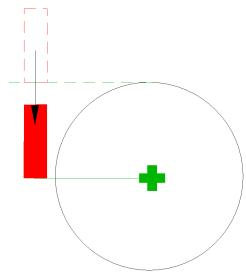
To zero the Z axis at the COR (green cross), move the cutter clear of the workpiece and zero the Z axis.
