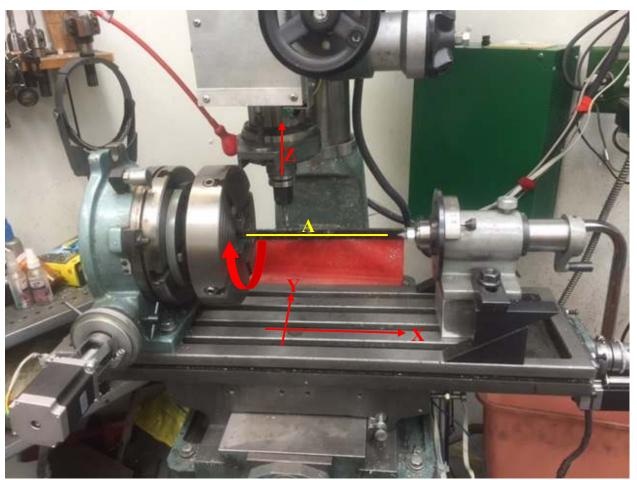
I needed to zero my Y and Z axes relative to the A axis Center Of Rotation (yellow) to within  $\pm 0.001$  inches. Here is how I did it.
