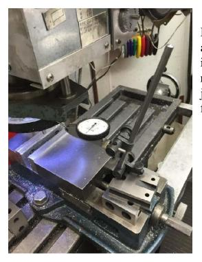
I can directly measure this backlash by using a finger Dial Test Indicator (DTI). The DTI is supported on the table and the finger is resting on the underside of the quill. Using just finger pressure, I can raise the quill a few thousandths of an inch.
