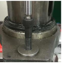
The piston's end sits in the top of a Socket Head Cap Screw 5/16-18 bolt which is threaded into a piece of cold rolled steel.
