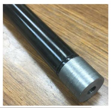
I drilled out a <sup>3</sup>/<sub>4</sub>" length of CRS using a #1 drill. It was then possible to screw the metric stud on securely.
