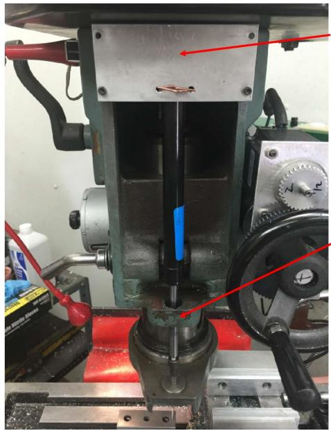
I happened to have an aluminum plate left over from a previous project. I used it and a length of copper wire to gently secure the top of the gas spring so it would not move off of the top support surface.
