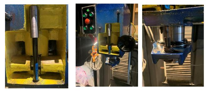
It provides about 100mm of stroke on the spindle under the cylinder pressure. Honestly I had no confidence using a slot drill/ uni mill before but with this mod it has completely changed. I have done one small job & a fairly large job last couple of days and it seems to have done the trick.
