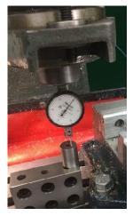
When I put down a spacer block "B" inches thick, I read a thickness of "A" DRO inches.
