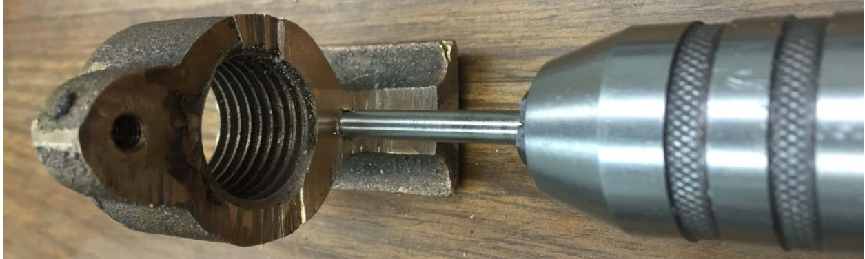
The body of the nut's hole was tapped 10-24.
