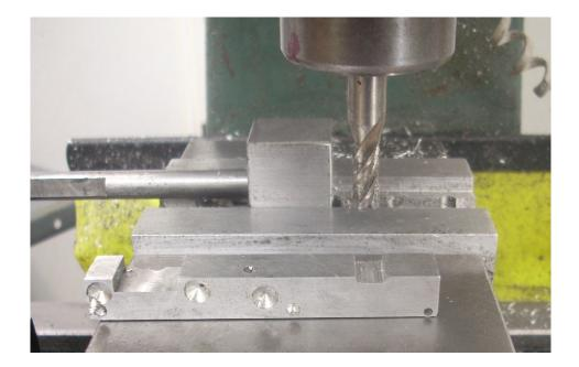
The block of aluminum resting on the vise was previously clamped in the vise jaws and a 0.075" deep slot cut by this end mill. The width of that slot is exactly how wide that end mill will cut when mounted in this collet and spindle when cutting aluminum to this depth. It is reasonable to assume that a heavier cut, a higher feed rate, and/or harder material will increase the effective end mill diameter. Beyond these caveats, long cuts can suffer from variations in the ways.
