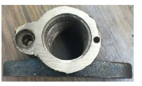
The first step was to drill a #36 tap hole at approximately the same height above the flange as the existing take up screw hole. Take care to position the hole so the screw head does not contact the leadscrew and the threads to be cut in this hole do not break out of the casting. It is best to drill using a drillpress to insure the bit does not tilt and break through the inner or outer walls of
