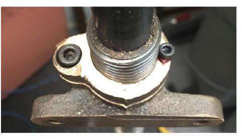
Here is the assembled modified nut on the X leadscrew. I used Loctite<sup>®</sup> Red on the threads of both screws. Then the screws were adjusted to give a sliding fit on the leadscrew.
