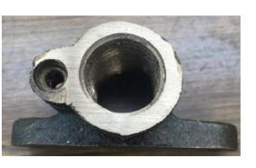
On the Y axis take up nut, there was plenty of room for the second screw so a 10-24 was used. But on the X axis nut, space is limited. We only have a wall thickness of about 0.2 inches. The largest screw that can fit is a 6-32. It has a close fit clearance hole of 0.1440 inches giving a wall thickness of about 0.028 inches. Ouch! That ain't much.
