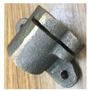
After drilling this tap hole, saw off the smaller section. Then open out the hole in the smaller part using a #27 for a close clearance. Run the tap through the hole in the larger piece.
