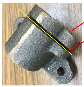
The X axis take up nut worked fine when new. But as it wore, the partially cut segment of this casting was bent over by the take up screw in order to reduce backlash and it fit the leadscrew threads worst and worst.
