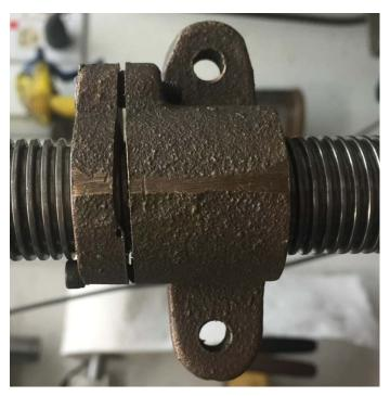
This side view shows how much the mounting holes and body of the casting are out of true with the major axis of the leadscrew. It really does not matter as long the leadscrew can be aligned with the X ways.
