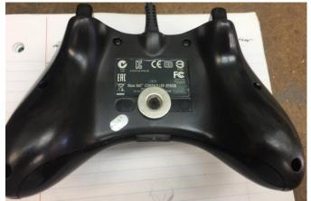
I had a neodymium disk magnet<sup>3</sup> with a countersunk center hole. By replacing a mounting screw with a longer one, the magnet was attached.
