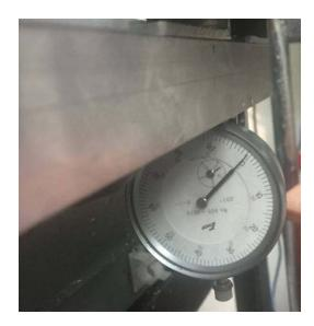
Moving to near the right bearing, we read out the difference in height.
