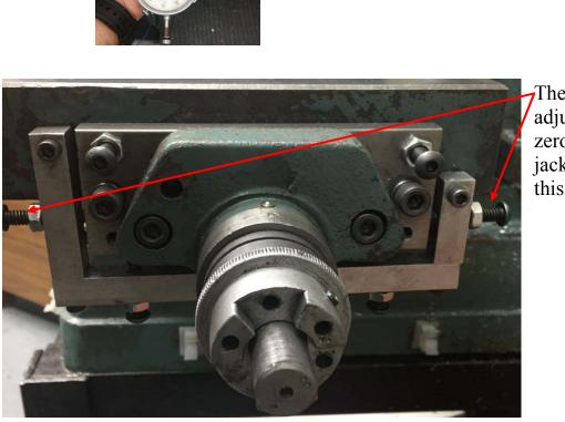
The horizontal jack screws are adjusted until the yaw equals zero. Then the loose horizontal jack screw is tightened to lock this position.
