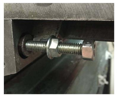
The key action here is to carefully adjust the X gib to be snug but without "excessive" drag and lock its position relative to the apron. See <u>http://rick.sparber.org/GR.pdf</u> for details of how I modified the locking mechanism.
