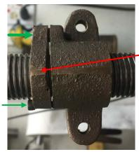
The first requirement, "The take up nut must be aligned with the leadscrew", is satisfied by using the modified take up nut. The adjustable part of the take up nut applies pressure axially to the leadscrew threads. This tends to center it due to the profile of the threads which are tapered. The original design put pressure only on one side which drove the leadscrew off center.
