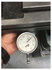
With the instrument near the left bearing, the DTI is zeroed.
