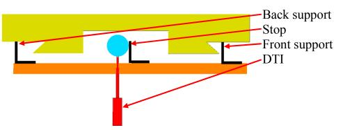
With the instrument in place near the left bearing, the DTI is zeroed.
