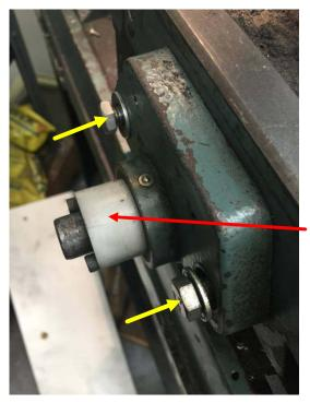
The left bearing support was badly worn after 25 years of half hearted lubrication. I saw about 0.02 inches of play between "bearing" and leadscrew shaft. This bearing was just a hole through the casting. Since I'm trying to align the leadscrew to within 0.0005 inches over its length, I cannot live with this much slop.
