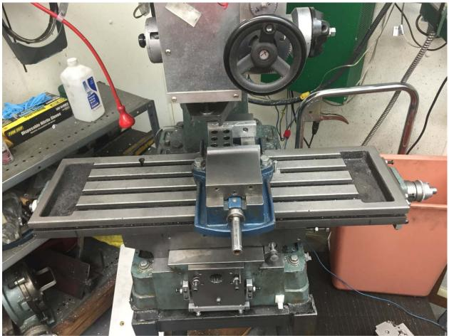
I was able to set the backlash to 0.002 inches at the left side of my vise. It rose, without binding, by 0.0004 inches after moving 4 inches away to the right side of the vise. About 0.0002 inches of this is radial leadscrew error which is cyclic as the leadscrew turns a full revolution.
