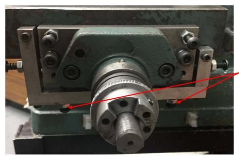
Then we use the vertical jackscrews to adjust the height of the right bearing until the DTI reads zero.
