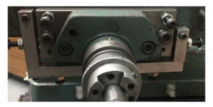
My solution was to make a new surface for the bearing block. This surface can be set at any small angle relative to the end of the table. In order to minimize deflection, the surface is made from  $\frac{1}{2}$ " steel.
