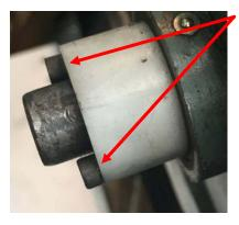
Two 6-32 screws were added to secure the plastic. The only force on this new bearing is the weight of the leadscrew so these small screws are adequate.
