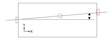
This instrument can tell us when we have zero yaw. When yaw is zero, the leadscrew is parallel to the XZ plane.
