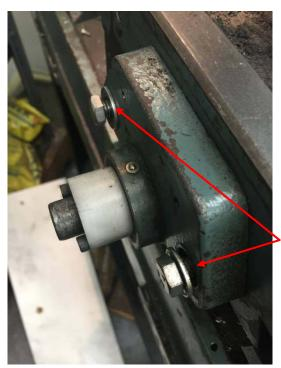
The take up nut is first tightly bolted to the apron and the leadscrew fed through until it enters the left bearing. This is loosely attached to the table. The right bearing is then loosely fitted.
