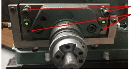
Two top screws plus two bottom set screws carry the force of the two mounting bolts (under the green dots). In this way, the mounting plate can be tilted as needed to follow the leadscrew.
