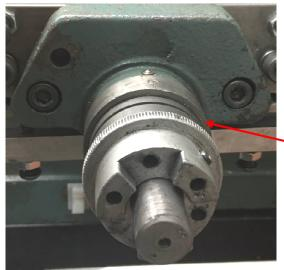
Inside the right bearing block are ball bearings that are intended to permit easy rotation of the leadscrew while preventing movement along the X axis. As manufactured, the leadscrew was able to slide in and out about 0.01 inches. The addition of a variable thickness washer let me preload the bearings and remove all but about 0.0001 inches of axial motion. This axial motion directly adds to my X axis backlash. See http://rick.sparber.org/VTW.pdf for details.
