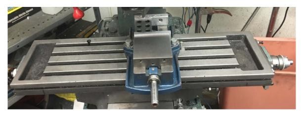
The RF-30 Mill/Drill uses a leadscrew and take up nut to move the table along the X axis (left/right movement). When converted to Computer Numerical Control, minimizing backlash in the leadscrew/nut arrangement becomes critical. It must also change as little as possible as the table moves. This is because the CNC software can cancel a fixed backlash but any deviation will become positional error.
