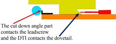
The horizontal flat part contacts a surface parallel to the ways to keep the instrument horizontal.
