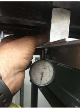
The pitch instrument is then zeroed on the leadscrew near the left bearing. Side view:
