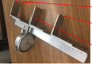
Note that the back support has been cut concave. This leaves just the corners to contact the far ways. The front support was cut with a point. In this way I have 3 points contacting the ways. As long as these 3 points are in contact, there will be perfect alignment with the ways and no rocking. I have a stop flanked by my DTI to align to the leadscrew and measure its surface. The end of the DTI's push rod has a large flat screw in it to bridge the threads.
