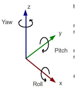
• Movement along the **X axis** - this is caused by bearing play and we can minimize it
