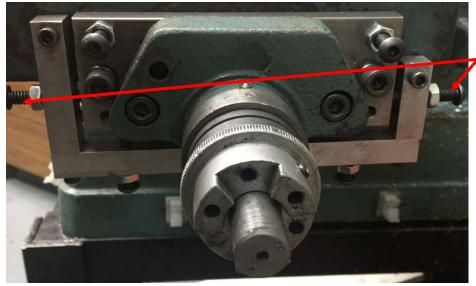
This end view of the right bearing shows a pair of jack screws that enable this motion. Loosen one and tighten the other.
