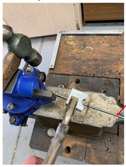
I'm holding the tool in a ViseGrip, which acts as a handle. A forming rod is lying on my anvil.
