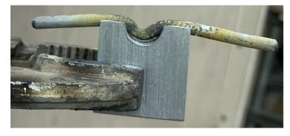
Holding the cross rod in pliers, I heated the center cherry red. Then, I laid it across the forming rod and put the tool on top. After two whacks with the hammer, I heated the rod again and repeated the process. The rod was then almost formed to the contour of the rod and tool.
