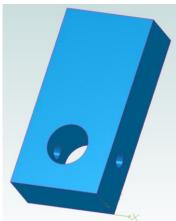
I designed the tool to fit 0.15-inch diameter steel wire. Since this is a one-off project, I used aluminum. CRS would hold up better after repeated strikes with the hammer.
