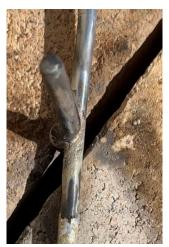
With the two rods closely fitting, I heated them to cherry red along with a speck of Harris Stay-Silv black brazing flux before introducing a small quantity of silver braze. The braze wicks into the tiny gap between rods for a strong joint. Since the contact area is filled with braze, this joint should be stronger than if I welded it.
