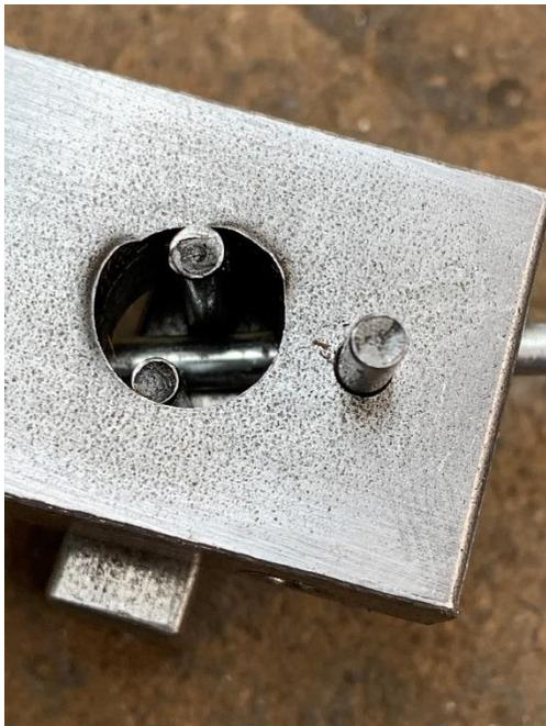
I drilled a hole in the arm that accepts both pins. In this way my arm pivots around two rather than one pin as it resists the bending force. I also flipped the arm over to insure that the wire pushes on the base of each dowels. That minimizes the bending moment.
