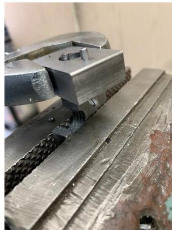
Here you can see how the arm pin clears the base due to the cut out. In the finished design, I'll just use a shorter block for the base.
