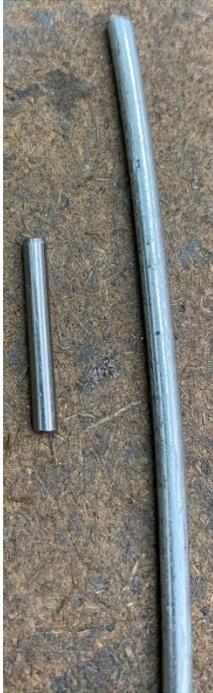
An appealing challenge was to bend some #7 gage wire (0.144" diameter) around a 1/8" diameter dowel pin. The benefit here is that the wire would then have an inside radius of only 1/16<sup>th</sup> of an inch.
