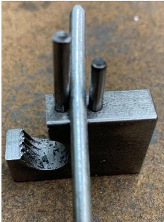
Here you see two dowels spaced a little wider than the diameter of my wire. This leaves no room for the arm that must pivot around one of the pins in order to form the bend. There is a method to my madness.
