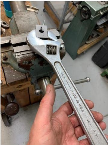
For this experiment I used a large adjustable wrench to turn the arm. The finished design will be made with a long bar of steel. The base is clamped into my bench vise.
