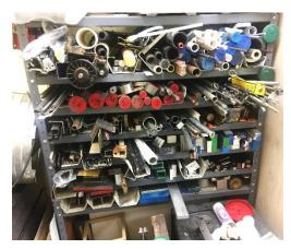
This is common metal shelving loaded with various U shaped trays. You get mostly random access and direct visibility as long as it is not overloaded. Those U shaped trays prevent sideways avalanches of metal. These trays are cut up plastic rain gutter.
