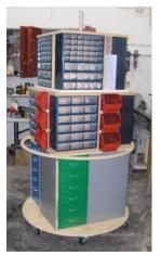
This masterful fastener storage unit was designed and built by John Herrmann. He has a large shop so this saves him steps. The fasteners have been organized so there is minimal turning of the unit during a job.
