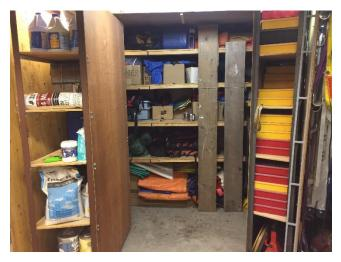
Dave calls this his layered storage area - 3 layers deep. First is the front of the hinged panels, with nominally "flat" stuff hanging (like ladders). Opening the panels reveals shelves. The shelving units are welded assemblies that are also "hinged" on wheel bearings to allow access to fixed shelves behind. The main reason for this extravagance (other than I thought it was a neat idea) is that the space was
