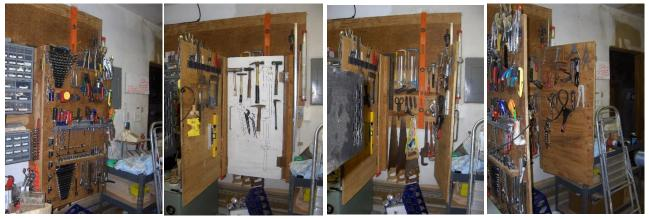
Here is a multilayer tool storage cabinet from John's shop. The cabinet has several doors with tools hung on each face. A little harder to see and access random tools but extremely good tool density.
