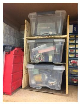
John and I got together and came up with a rack to allow random access for the tubs inside my cabinet and atop my cut offs rack. We used some 3" x 3" cardboard angle stock that John had recently found. Being wider than the usual stock, it did a good job of supporting the narrow bottoms of the tubs, while providing clearance for the wide tops.
