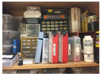
OK, mostly bad here. The fundamental problem is that the cabinet is deep. Plastic drawer units have been pushed to the back. The space in front is, at best, wasted. At worst, it becomes a collection point for material waiting to be put away. The compromise was to place boxes in this space.
