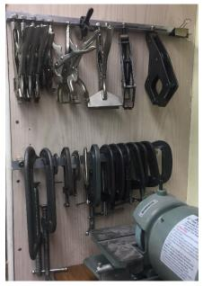
The Vise-Grips can be left in the open position and the C-clamps are held as long as they are partially open<sup>3</sup>.
