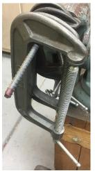
To keep the C-clamps from falling off the rod, they must first be closed all the way. Yet, to use one, it must be opened. Therefore, this storage method forces us to have all clamps in a non-ready state.
