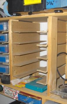
Here is another option from John Herrmann. Those pieces of angle stock are compressed cardboard which are glued and nailed to 1x2s. The angle stock is commonly found as packing on heavy items like washing machines.
