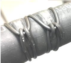
The loop is a bit wide because my tool is wide. I think I could remake the body of the tool using 1/8 inch thick CRS which would help a lot here. If the body was thinner, the cross drilled holes must be moved in too.
