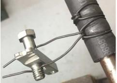
I then turned the bolt backwards about half a turn and slide it off of the wires.
