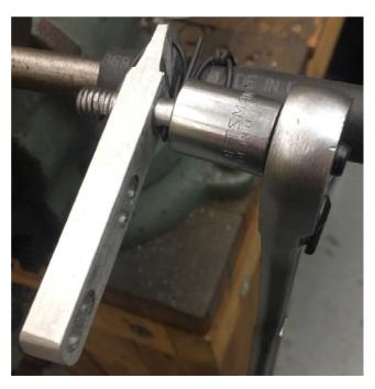
I first turned the bolt by hand to wrap the wires around its shank. Then came the large force. Care must be taken while turning the bolt with the socket wrench. I could easily snap the wire.
