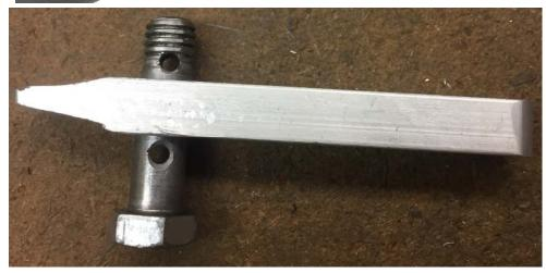
Another minor improvement would be to screw an acorn nut on the end of the bolt so it doesn't separate from the body. The threads are badly chewed up but they will hold a nut snug.
