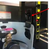
The safety bar is loosened and lowered onto the collar. Once the wing nut is tightened, the tank is safely captured. Not shown is that I had to remove that black spacer above the hole.
