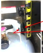
The scale has a hook on it that supports the tank. The platform was sized to put the tank near the hook position when full. Note that the hook is above the hole in the collar.
