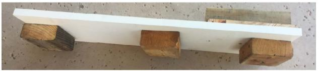
The platform was made from a scrap shelf about a 1/2 inch thick, 8 inches wide, and 20 inches long. Three blocks of 2 by 4 were screwed into the bottom. The top has a longer piece of 2 by 4 and a piece of 5/8 inch thick plank.
