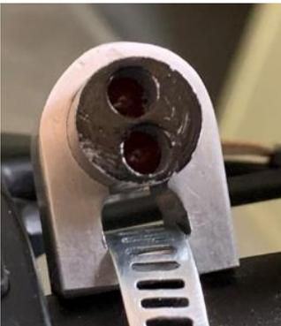
The result is displayed on two red LEDs mounted on my handlebars. This scheme tells me the State Of Charge with a precision of  $\pm 5\%$ . While far from perfect, it is an improvement over measuring voltage.
