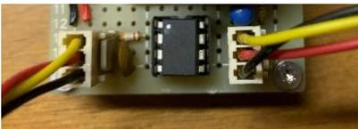
My solution is to add a [small computer](#) that measures the current once per second and subtracts it from the initial ampere-hour value.
