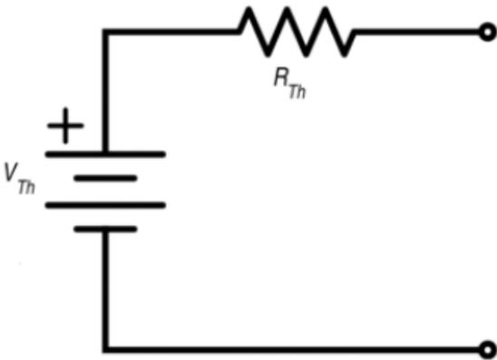
A battery can be modeled by an ideal voltage source,  $V_{Th}$ , and an ideal resistor,  $R_{Th}$ . When no current flows, the voltage measured at the terminals will equal  $V_{Th}$  because there is no voltage drop across  $R_{Th}$ . As the current increases, more voltage is dropped across  $R_{Th}$ , so the measured voltage drops. All of this happens while  $V_{Th}$  remains unchanged.
