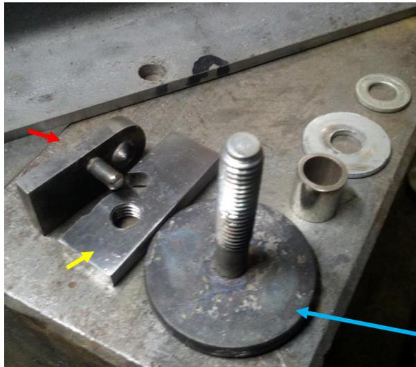
The guide (red arrow) is a sliding fit in the table slots. Its rounded end prevents jamming as it slides towards the center of the table.
