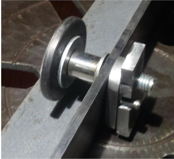
The lock is custom-made to fit my drill press table. I drop it into one of the four radial slots, turn the knob about half a turn, and the fence is secure.
