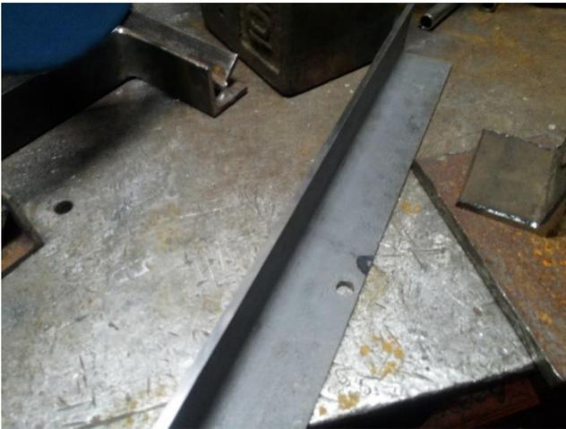
The bar is a piece of angle stock with a hole drilled into it to accept the locking mechanism. It was selected to be straight and smooth.
