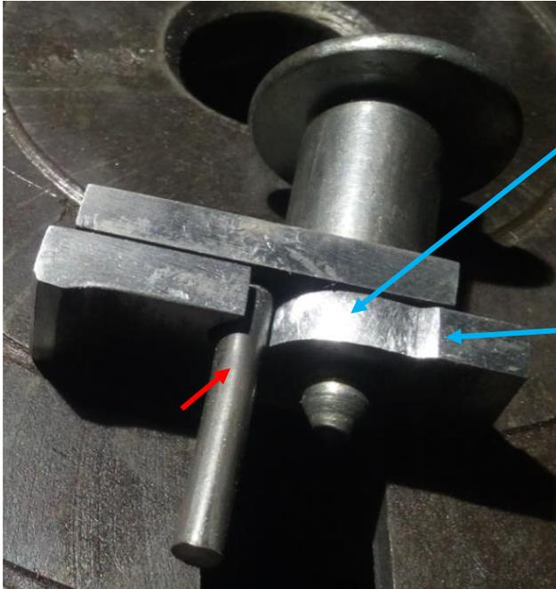
The locking bar has a complex cut in it. In the unlock position, the rod (red arrow) prevents the locking bar from rotating too much. As the bar rotates into the lock position, the rod travels an arc until it hits this stop.
