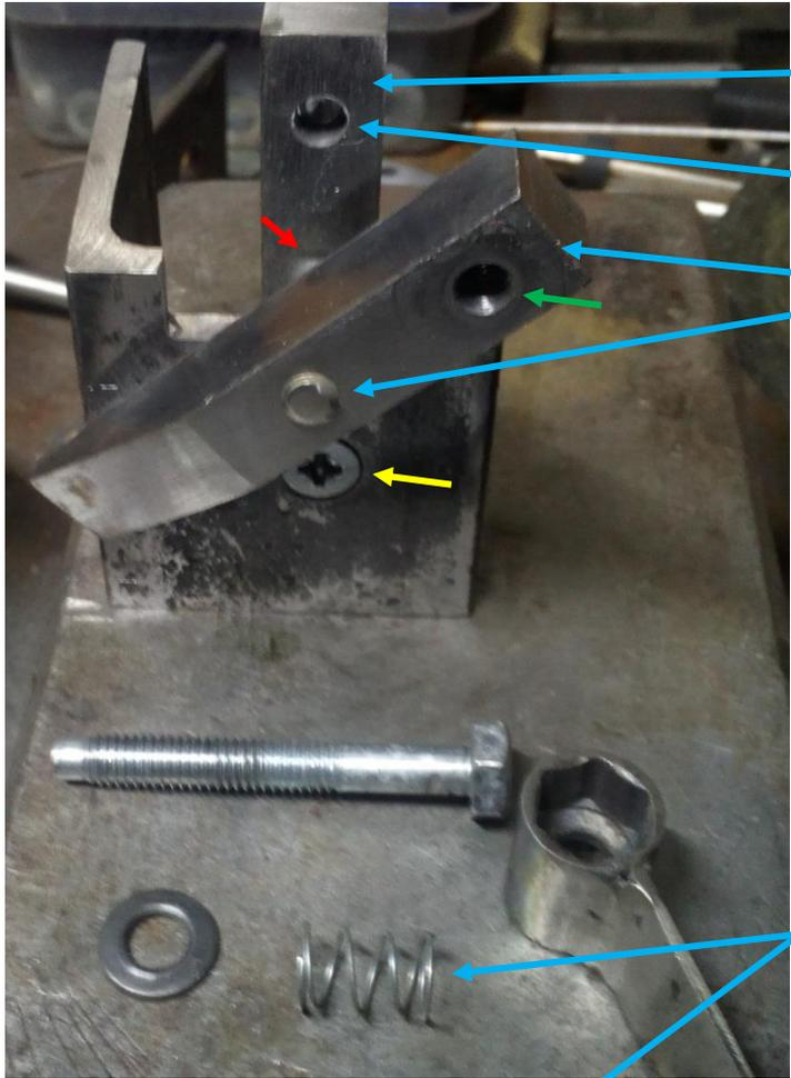
The clamp consists of two bars. The rear bar is secured to the stop (yellow arrow) and has one threaded hole (red arrow) and one blind clearance hole.
