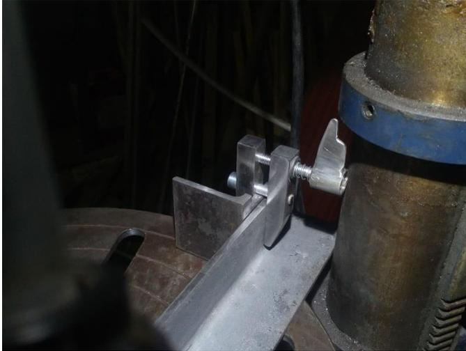
The adjustable stop can be positioned anywhere along the bar and then locked in place.
