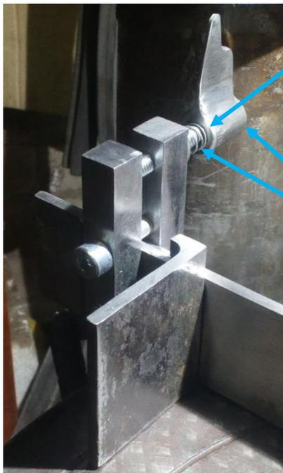
The handle has a hex recess that mates with the hex bolt occupying the top holes. The handle can be repositioned during tightening and then removed if it is in the way.
