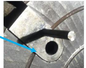
The pivoting lock (yellow arrow) is narrow enough to pass through the slot. When it rotates 90°, the lock is secure.
