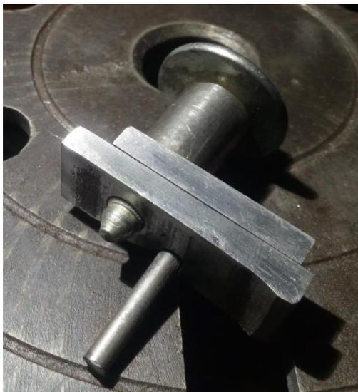
Here is the partially finished lock. With the guide and locking bar in alignment, they can drop through a slot in the table. I did have to file the slots, so they have a uniform width.
