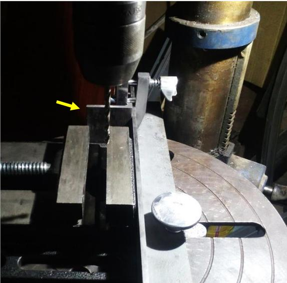
A fence permits me to drill a series of holes all on the same line. The stock is secured in my drill press vise, which is pressed against the fence. I can then slide the vise along the fence.
