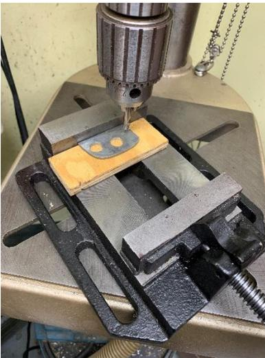
But in this case, my movable jaw cannot reach the stock because my scrap of wood is too wide. Now, I could cut the wood to be narrower but this will also weaken it. I prefer a solution that doesn’t require constantly cutting bits of support wood. Besides, I’m always looking for new ways to do old things.
