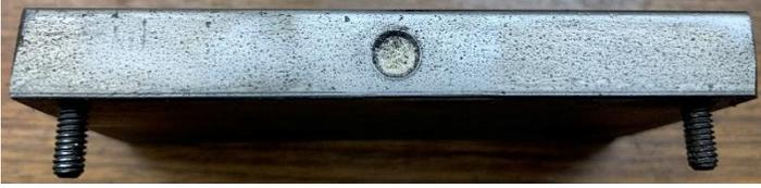
John Herrmann suggested adding magnets to the edge in contact with the movable jaw. I found that a single 1/8 inch thick, 1/4 inch diameter neodymium magnet was sufficient to keep the extension jaw
