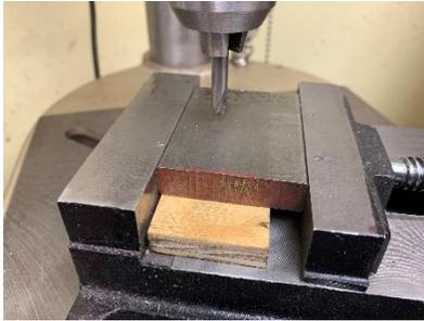
Say I wanted to drill a hole in this piece of stock and not “tag” my drill press vise. It is common practice to place a piece of wood under the stock. The wood must be strong enough to resist the downward force, wide enough to provide stability yet narrow enough to allow the movable jaw to contact the stock. All that is true here.
