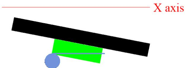
If the vise is out of alignment, the cutter will still follow the X-axis but the stock will be cut into a taper.
