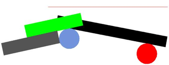
X axis I can erect a bar (green) that hangs over the vise. It is tangent to the blue circle. Then I can clamp a block (gray) to this bar that also touches the blue circle. The angle of the green and gray bars doesn't matter.
