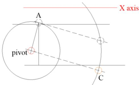
What if I tracked a new point, call it C that has the same offset? Ah, C is on a line that passes through my new pivot point so I'm back to my original configuration. I can measure my new pivot point distance and then only focus on point C.
