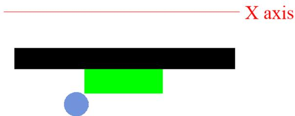
The black rectangle is the fixed jaw on my ideal vise. Clamped to it is a piece of stock. The circle is my end mill. As the end mill moves across the face of the stock, it will cut a face that is parallel to the X-axis.
