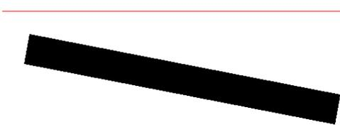
X axis It is time to return to my misaligned vise. We now understand that the easiest way to align the vise jaw is by first picking a pivot point on its face. Then rotate the vise until a second point, on its face, is at the same distance.
