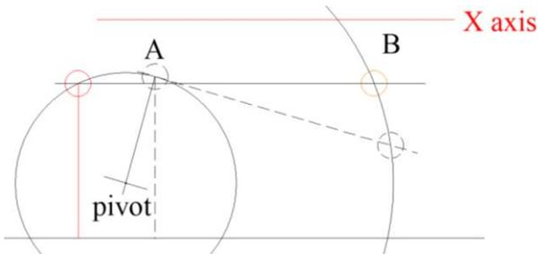
If I chose a pivot point, not on my vise jaw, the distance from it to my reference line would change as I rotated the vise. Compare the dashed vertical line to the red vertical line. This means I must move back and forth between A and B to know when they were equal. This is a royal PITA.
