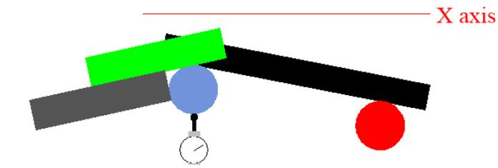
I secure a finger Dial Test Indicator (DTI) to my spindle so it touches the pivot rod. Then I move the table along the X-axis and watch the needle rise and fall as it passes the rod's centerline. I record this value.
