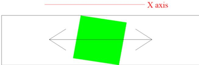
In reality, nothing is straight or parallel. If I tried to tighten the gib too much, it will bind up and the table will lock. Typically, this will happen at one or more points in the table's travel. The only solution is to back off on the gib and permit more play.
