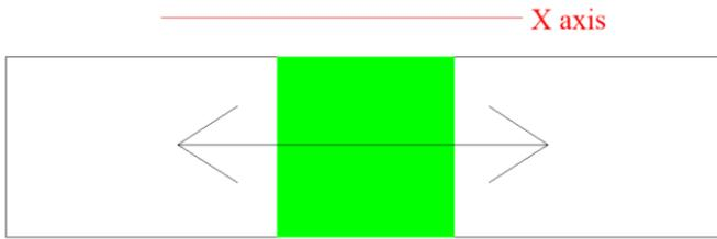
The table slides on ways, represented by the green square and the top and bottom lines of the black rectangle. If all surfaces are perfectly straight and parallel, the ways can be adjusted via a gib for perfect movement.
