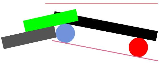
X axis I can draw a line, tangent to my blue and red circles. When this line is parallel to the X-axis, my vise jaw must also be in alignment.
