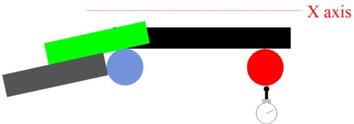
I gently pivot the vise while keeping the blue pivot bar touching my green and gray bars and stop when the DTI reads the recorded value. I then move the DTI back and forth along the X-axis over the red bar to verify I'm still at the maximum deflection since the pivoting does cause some X-axis movement of the rod relative to the spindle. The vise's fixed jaw is now parallel to the X-axis.
