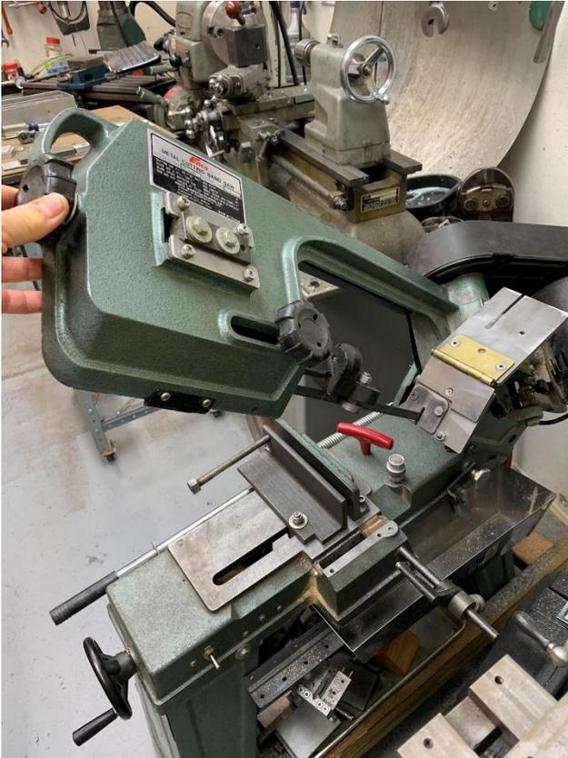
My heavily modified Enco Horizontal/Vertical bandsaw has a [flip-down table](#) which I use when the saw is in the Vertical position.
