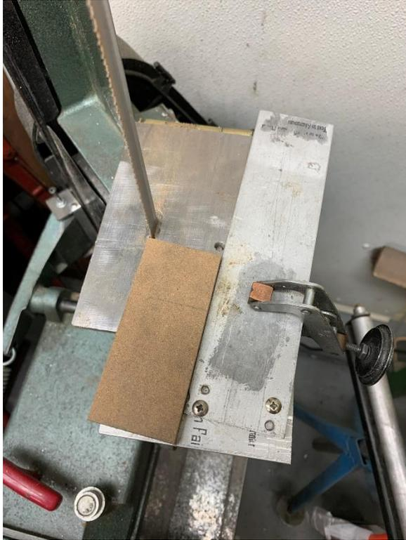
To use my fence, I first make contact between the guide and the front edge of the table. Then I slide it over to the desired distance. And finally, I clamp the fence down.
