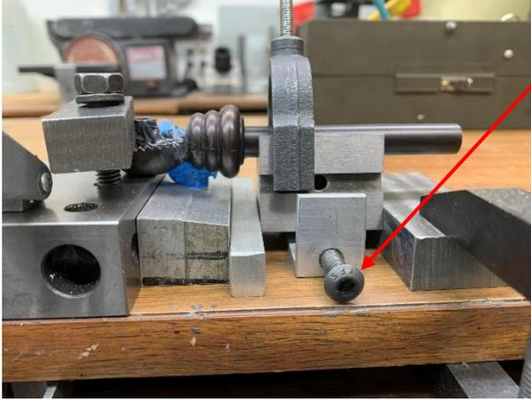
The solution can partially be seen here. Turning the button head screw pivots the V block which changes the altitude of the shaft.
