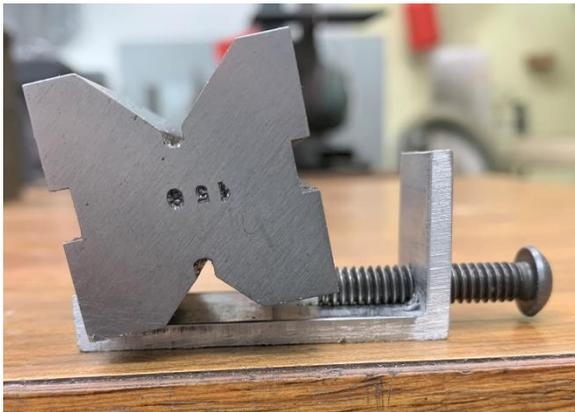
Nothing fancy about the attachment. It is just a scrap of aluminum channel cut down on one side and drilled/tapped on the other.
