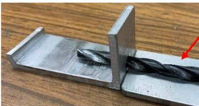
I drilled the tap hole by first laying down a piece of aluminum that was the same thickness at the channel. Then I rested the drill on top of this scrap and drilled into the vertical part of the channel. After applying the 1/4-20 tap, I ran the screw in and it rested on the inside surface of the channel.
