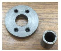
I found a piece of gas pipe that almost fit through the bore. It was turned down to a sliding fit and used to align the drive spline and drive collar. I punched a small feature into the outside diameter of the drive collar to line up with a punch mark on the drive spline. This was helpful during installation. Offset the punch marks so the correct face of the drive collar is forward.
