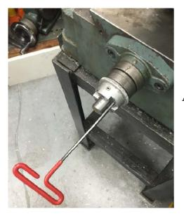
Access to the set screws is through the drive spline.
