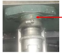
One source of backlash and change in backlash as a function of table position on a RF-30 Mill/Drill is the play in the bearings<sup>2</sup>. Adding shims certainly helped but it was difficult to get exactly the right thickness and also be able to drive the locking spring pin through the drive spline.
