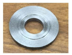
I started with a round piece of  $12L14 \ 1-3/4"$  in diameter. The center was bored out to 0.668 inches to match the bore of the drive spline . You are looking for a sliding fit. The depth was around  $\frac{3}{4}$  inch.
