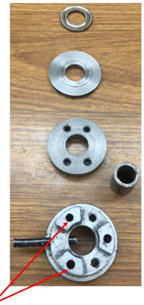
the outer bearing surface which directly contacts the outer ball race
