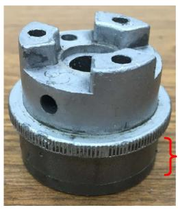
The driven spline seems to be made from a cast zinc-aluminum alloy. Holes are cast into the spline lands that go in about 0.2 inches.
