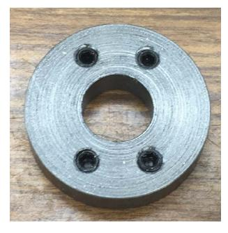
Then the drive collar was removed and I used a #7 drill to drill through the drive collar in four places. These holes were then tapped  $\frac{1}{4}$ -20.
