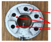
Select a drill that is a sliding fit to one of the cast holes. Using a drill press or your mill/drill, drill two holes centered on the small cast features plus drill out the holes in the spline lands.
