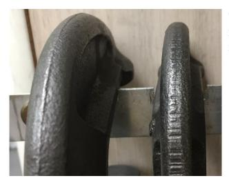
The two C clamps on the left were rather large and heavy. They tend to rotate so I cut notches for them.
