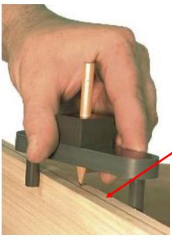
If you wanted to make a tool that finds the centerline of a rectangular solid, take a bar and drill three holes with equal distance between centers all on the same line. Install pins in the outer two holes. By rotating the bar so the pins contact the flanks of the rectangular solid, that center hole will be on center. You can then put a scribe or marker in the hole and pull the tool along the longitudinal axis.
