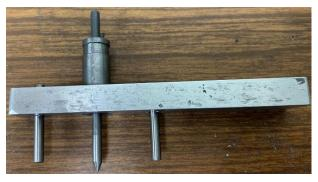
Replace the pencil hole with a 3/8-inch rod about 1-inch long. This will be our pivot. Drill a hole through this rod to accept a 1/8-inch pointed rod about 2-inches long. It will be our "spud". The adjacent holes are 1/8-inch and accept 1-inch long dowel pins. You can stake the pivot and pins in place or use Loctite. It is essential that the distance between holes is the same and that all three holes are on the same line.
