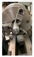
The washer will be a little under 1 inch in diameter, so I chucked up some 6061-T6 aluminum and faced the end square.
