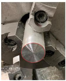
If you don't cut the grooves, you will find that the glue sets up at the perimeter of the aluminum bar as a thin line. This prevents air from reaching the rest of the glue, so it will remain uncured.
