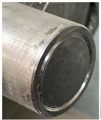
I placed the shim over the grooved surface and applied pressure with my tailstock-mounted drill chuck.
