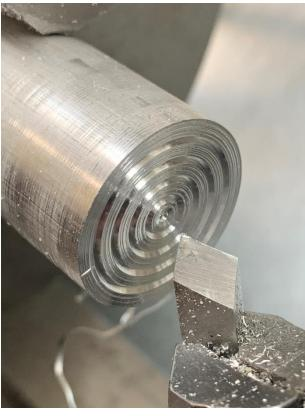
Now for the cool bit – I cut a series of grooves in the face. Since I planned to publish this trick, I made it pretty. The groves were spaced 0.1 inches apart on radius and 20 thou deep. It doesn't have to be this precise. The goal is to have grooves flanking raised, flat areas. I then used alcohol to degrease the face plus the surface of the shim stock square.
