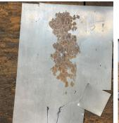
I started with a sheet of 15 thou shim stock. After cutting a 1-inch square, I used my ball peen hammer to roughly flatten it on my anvil.
