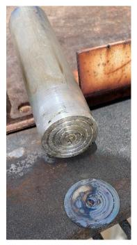
This next step is essential, take the aluminum bar with the shim attached *OUTSIDE*. The fumes released from heating cyanoacrylate glue can be dangerous.
